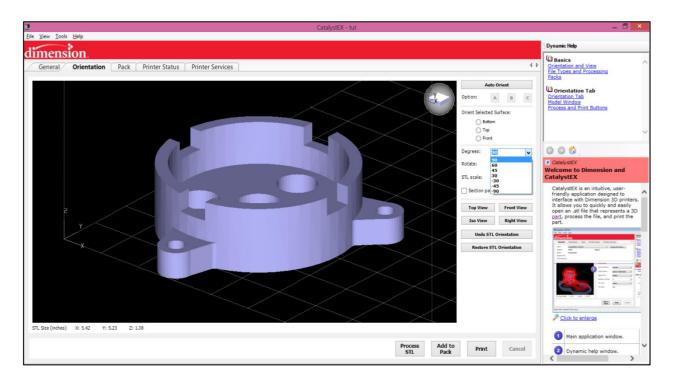
Figure 4.7 selection of manual orientation at diff. degree
