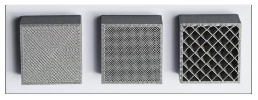
Fig. 3.3 (A) solid (B) sparse high density (C) sparse low density
