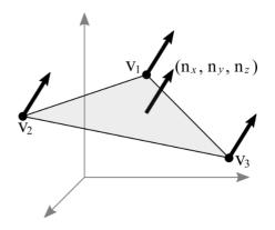
Fig. 2.2- A facet object with three faces and three vertices
