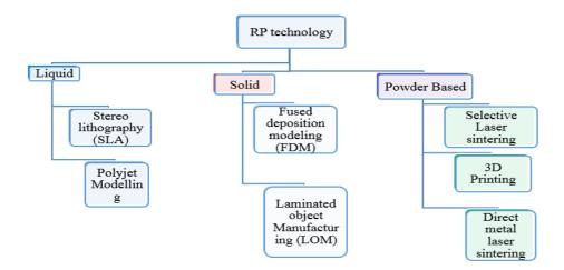
Fig. 1.6 Classification of Rapid Prototyping Systems
