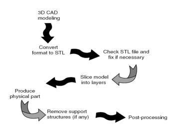
Fig. 1.5 Data Flow of the Basic RP Process
