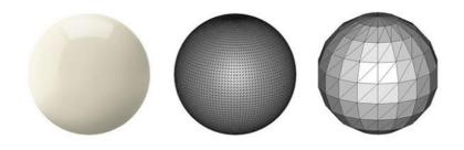
Fig 2.3 - Effect of degree of approximation in tessellation on Solid geometry
