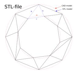
Fig. 2.1 - CAD Representation of a torus
