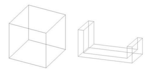
Fig. 1.1 Wire frame model
