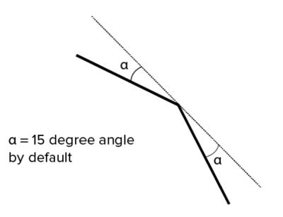
Fig 2.5- Angular tolerance (Angle between the normal of adjacent triangles )
