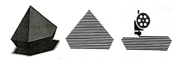
Figure 7.1 slicing of solid model
