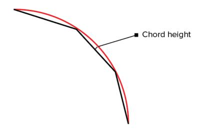
Fig 2. 4 - The chord height (height between the STL mesh and the actual surface)
