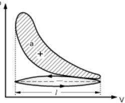
Fig. 5. 2 Indicator diagram
