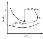
Fig. 5. 16 Performance curve for SI and CI engine at constant speed
