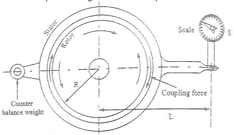
Fig. 5. 2 Principle of a dynamometer
