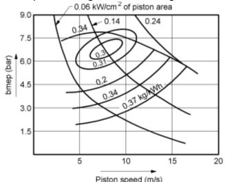
Fig. 5. 19 Performance map of a S.I. engine
