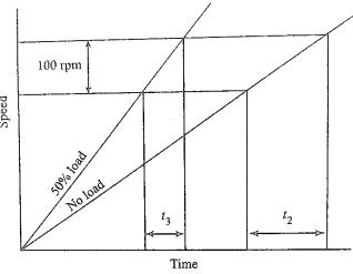
Fig. 9. 9 Graph for Retardation Test
