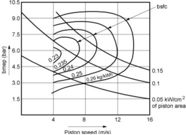
Fig. 5. 20 Performance map of a C.I. engine
