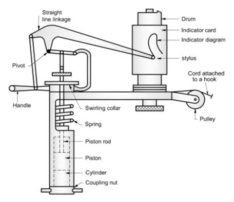
Fig. 5. 1 Engine indicator (Mechanical type)
