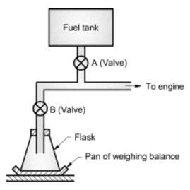
Fig. 5. 11 Direct weighing of fuel flow
