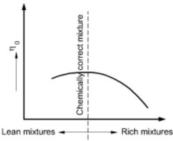
Fig. 5. 17 Brake thermal Vs Mixture strength
