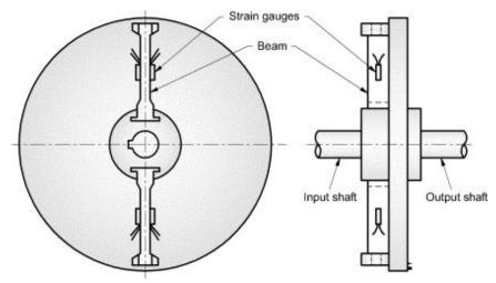
Fig. 5. 7 Transmission dynamometers
