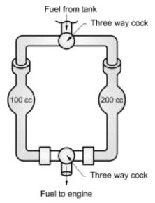
Fig.5.10 Volumetric Type Fuel Flow meter
