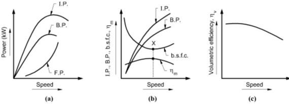
Fig. 5. 14 Performance curve for S.I. engine
