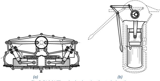
Fig. 5. 21 (a) VCR engine by changing the stroke length (b) Variman VCR engine using movement of crank shaft
