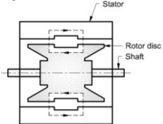
Fig. 5. 6 Eddy current dynamometer
