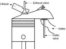
Fig. 7. 17 F-head combustion chamber
