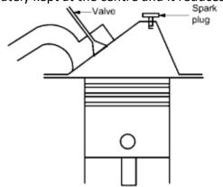
Fig.7. 16 Wedge head combustion chamber
