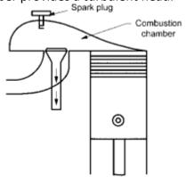
Fig. 7. 13 Recardo turbulent combustion chamber
