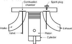
Fig. 7. 11 T-head combustion chambers
