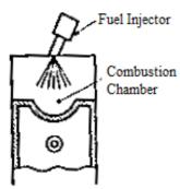
Fig.7. 28 M.A.N. combustion chamber
