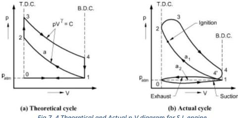
Fig 7. 4 Theoretical and Actual p-V diagram for S.I. engine
