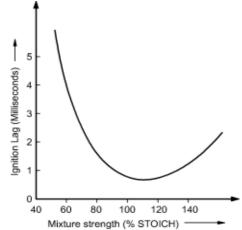
Fig. 7. 5 Effect of A/F Ratio on Ignition Lag
