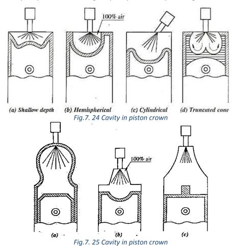
Advantages and disadvantages of this type of combustion chambers are as follows:
