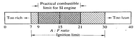
Fig. 7. 1 Ignition Limit Hydrocarbons
