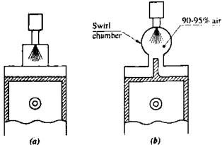
Fig. 7. 27 Turbulent or Indirect Injection (IDI) Combustion Chambers
