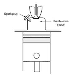
Fig.7. 14 Bath tub combustion chamber
