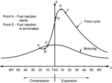
Fig.7. 19 Combustion stages in C.I. Engines
