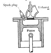
Fig.7. 15 Rover Head Combustion Chamber
