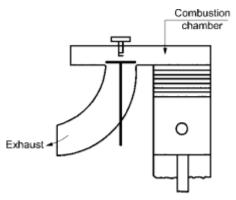
Fig. 7. 12 L-head combustion chamber
