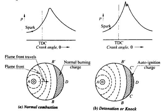
Fig.7. 9 Normal combustion and detonation
