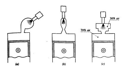
Fig. 7. 26 Precombustion chamber
