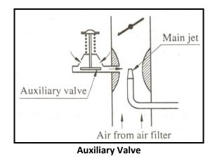
An auxiliary valve carburetor is illustrated in fig. With an increase of engine load, the vacuum at the venturi throat also increase. This causes the valve spring to lift the valve admitting additional air and the mixture is prevented from the becoming over - rich.
