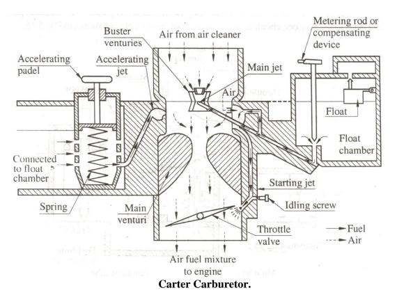
Idle and low speed circuit: For idling rich mixture is required in small quantity. In idling condition throttle valve (8) is almost closed. The whole of the engine suction is applied at the idle port (9). Consequently the petrol is drawn through the idle feed jet (10) and air through first bypass (11) and a rich idle mixture is supplied. In low speed operation the throttle valve is delivered both by the main venture and low speed port (12) through idle passage.
