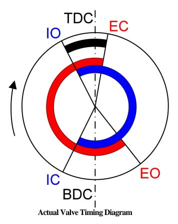
The Actual Valve Timing Diagram has slight variations with respect to the Theoretical Valve Timing Diagram. The variations are made in order to maximize the engine performance.
