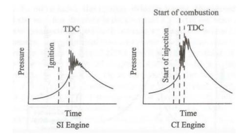
Detonation in the SI engine compared with knocking in the CI engine
