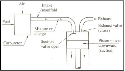
Charge transfer from carburetor to cylinder
