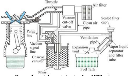
Evaporative emission control system for a MPFIengine
