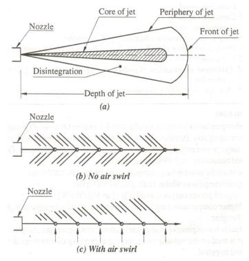
Schematic representation of disintegration of fuel jet in CI engine
