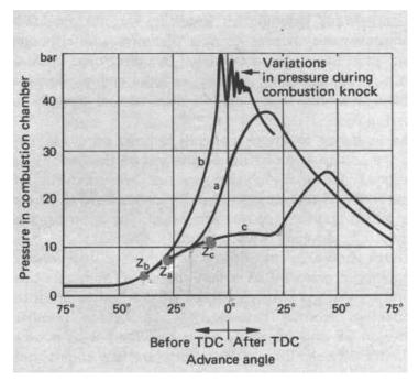
With optimum spark setting, max pressure occurs at about 15 degrees CA after TDC (10 - 15), half the charge is burned at about 10 degrees CA after TDC.
