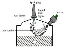
Schematic of a Stratified Engine Combustion System
