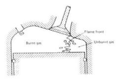
speed and peak pressure is obtained at 5 - 20 OCA ATDC. This is essential for max thermal efficiency. Since combustion takes a finite time, mixture is ignited before TDC, at the end of compression stroke – spark advance The second stage continues until maximum pressure is obtained and lasts about 25 - 30 OCA.
