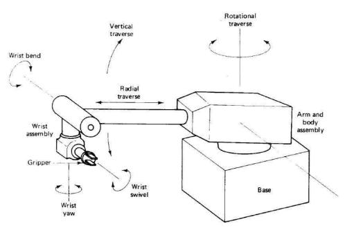
Figure 5.6 Typical six degrees of freedom in robot motion
