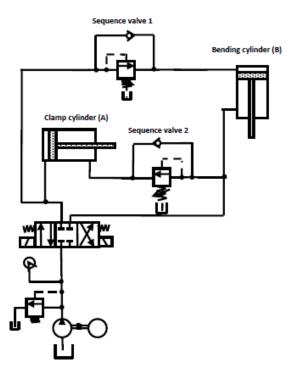
Figure 3.1 sequential circuit
