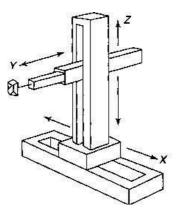
Figure 5.1 Typical Motions of a Cartesian or Rectilinear Robot
