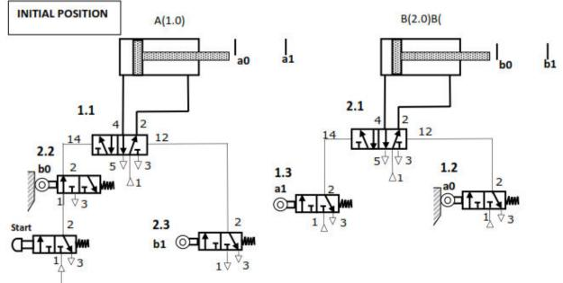
Fig. 2.1 Sequential operation of two double acting cylinders
