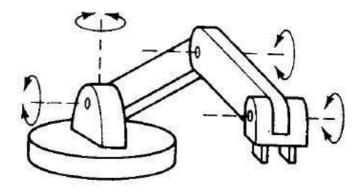
Figure 5.4 Typical Motions of a Cylindrical Robot
