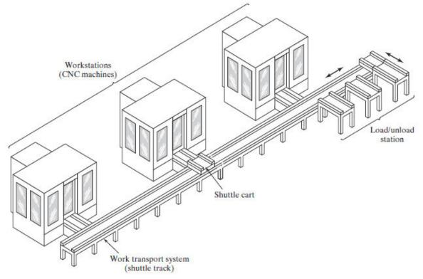
Figure 4.3 A flexible manufacturing cell consisting of three identical processing stations (CNC machining centres), a load/unload station, and a parts-handling system
