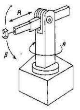
Figure 5.3 Typical Motions of a Spherical Robot
