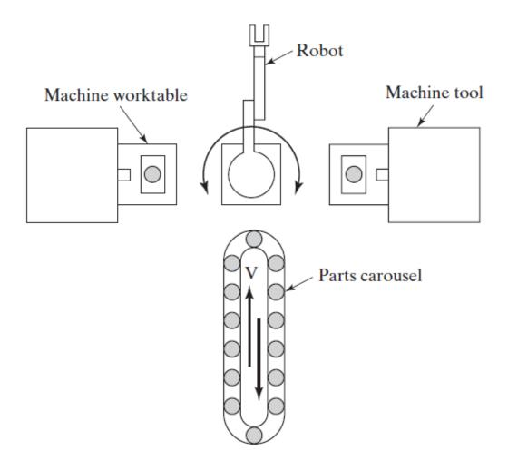
Figure 4.1 Automated manufacturing cell with two machine tools and robot.
