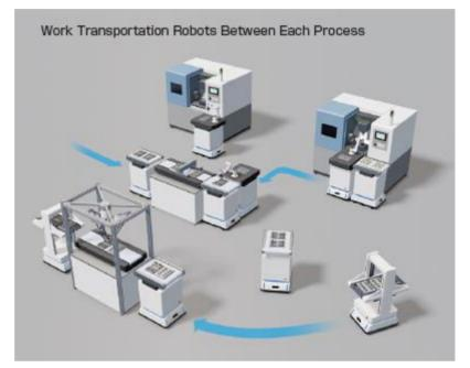
Semi-mobile modular automation lines have certain modules fixed to the floor. However, by integrating mobile robots with certain conveyor modules, mobile parts transfer becomes possible, and production efficiency can be improved by eliminating the manual transfer of parts between different process stations. A mobile robot with a small turning radius can work in a limited space and improve space efficiency.
