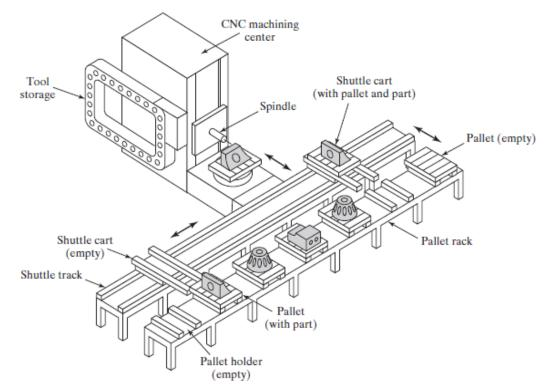
Figure 4.2 Single-machine cell consisting of one CNC machining centre and parts storage Unit
