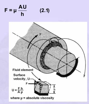
Fig. 2.2 Laminar flow of fluid in clearance space
