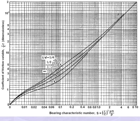
Fig. 2.11 Chart for coefficient of friction variable.
