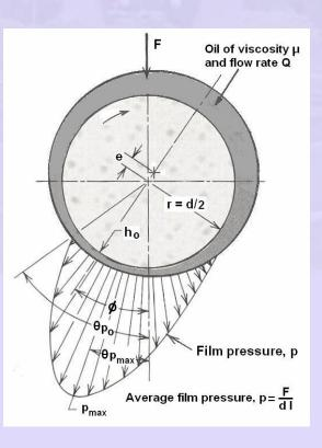
Fig.2.10 Stable hydrodynamic lubrication
