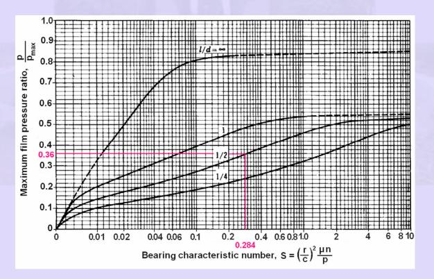
Fig. 2.14a Chart for determining the maximum film pressure
