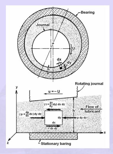
Fig.2.5 Pressure and viscous forces acting on an element of lubricant. Only X components are shown
