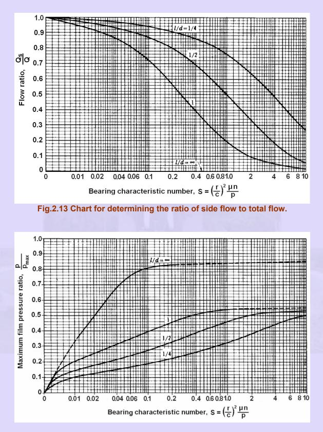
Fig. 2.14 Chart for determining the maximum film pressure.
