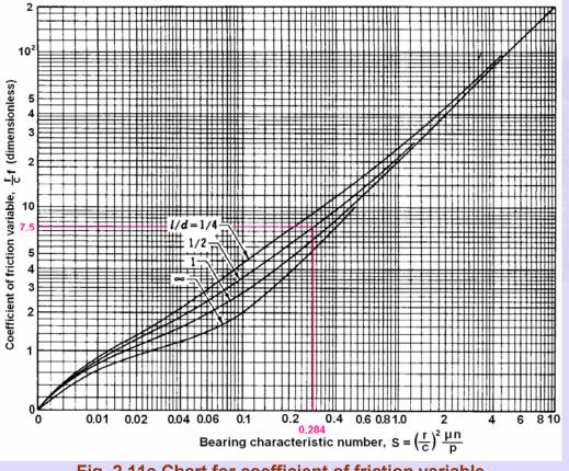
Fig. 2.11a Chart for coefficient of friction variable
