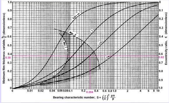
Fig.2.8a Chart for minimum film thickness variable and eccentricity ratio. The left shaded zone defines the optimum  $h_o$  for minimum friction; the right boundary is the optimum  $h_o$  for maximum load
