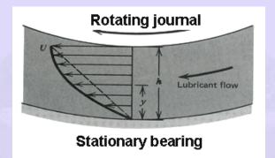
Fig. 2.7 Velocity gradient in the oil film
