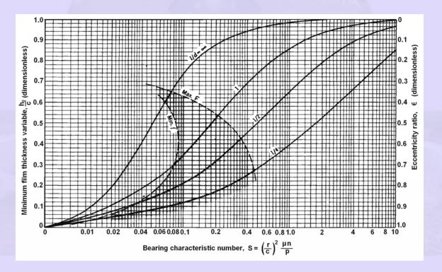
Fig.2.8 Chart for minimum film thickness variable and eccentricity ratio. The left shaded zone defines the optimum  $h_o$  for minimum friction; the right boundary is the optimum  $h_o$  for maximum load
