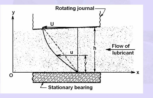
Fig. 2.6 Velocity distribution in the oil film
