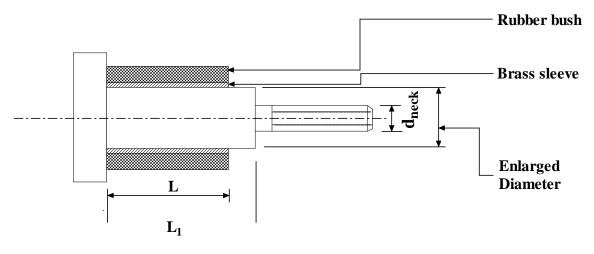
**5.2.3.1F-** A typical pin for the bushings.
