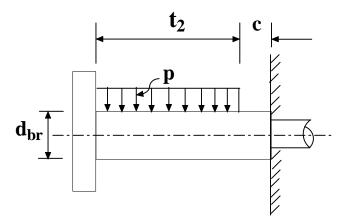
**5.2.2.2F**- Loading on a pin supporting the bushings.
