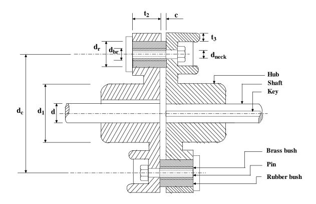
**5.2.2.1F-** A typical flexible coupling with rubber bushings.
