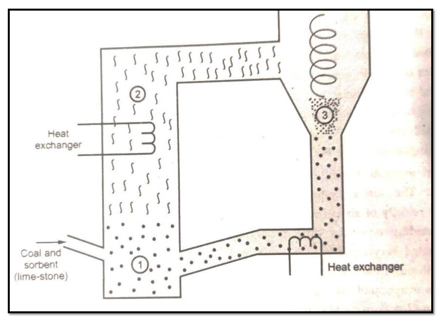
Circulating Fluidized Bed Combustion System(CFBC)
