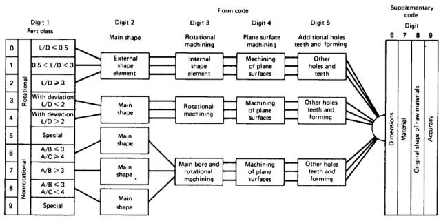
Fig.4.5 - Basic structure of the Opitz system
