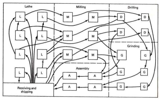
Fig.4.3 - Process-type layout
