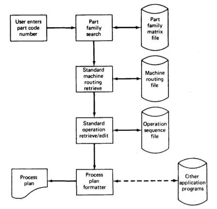
Fig.4.9 - Information flow in a retrieval-type computer-aided process planning system
