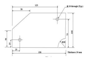
32. Prepare CNC milling part program for figure 1. (Thickness of plate is 15 mm)
