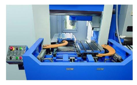
Machining Center with Pallet changer
