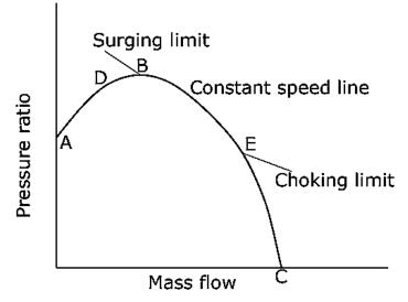
Fig. 10.8 Performance Curve of Centrifugal Compressor
