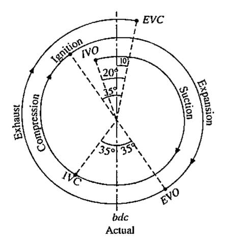
Fig. 7.2 Valve timing of 4 stroke petrol engine
