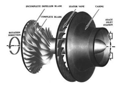
Fig. 10.7. Constructional details about centrifugal air compressor.
