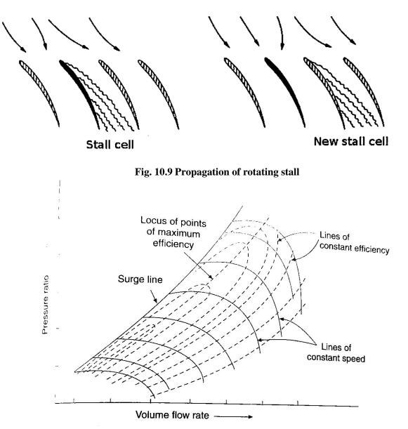
Fig. 10.10 Performance curves for centrifugal compressor
