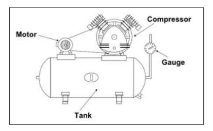
Fig. 10.1. Layout of reciprocating air compressor test rig
