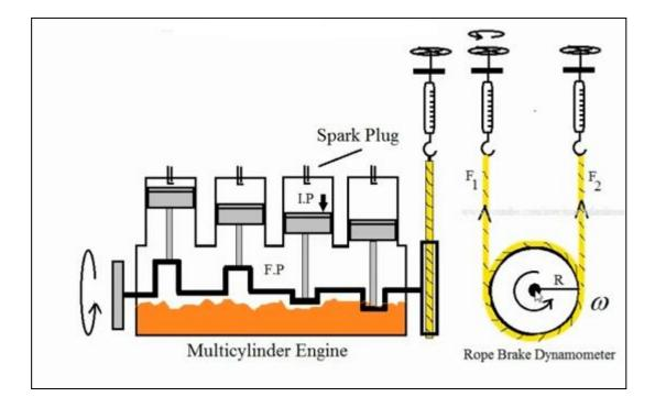
Fig. 9.1 Schematic layout of multi cylinder petrol engine test rig
