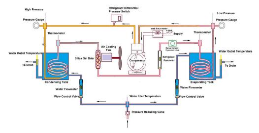
Fig. 5.1. Layout of heat pump system.
