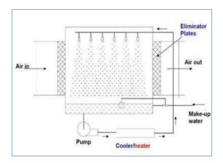
Fig. 6.2. Working of air washer.
