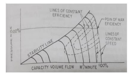
Fig. 10.6. Axial flow compressor characteristic curve.
