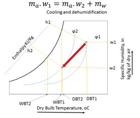
Fig. 2.5. Cooling and Dehumidification process
