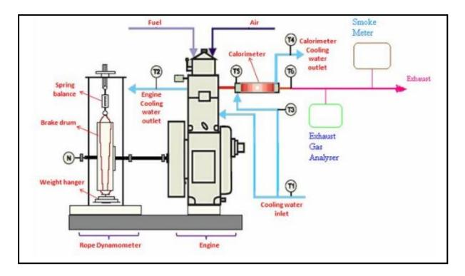
Fig. 8.1 Schematic layout of diesel engine test rig
