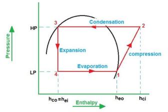
Fig. 5.2. Plot the operating cycle on p-h chart.
