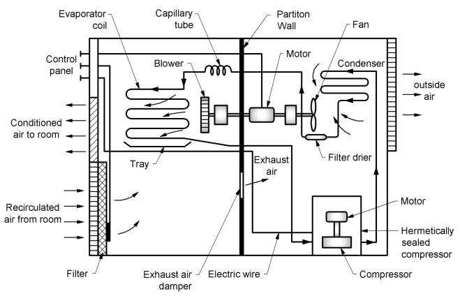
Fig. 3.1. Layout of window air conditioner.
