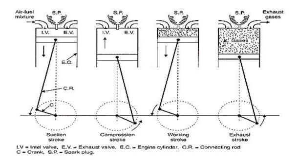
Fig. 7.1 working of 4 stroke petrol engine
