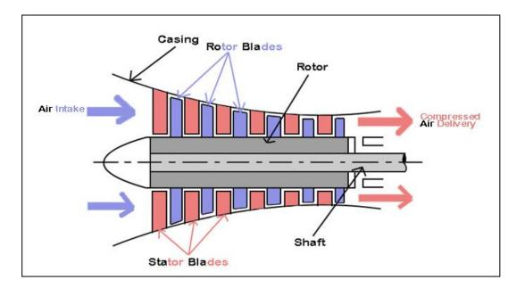
Fig. 10.5. Schematic layout of axial flow compressors.
