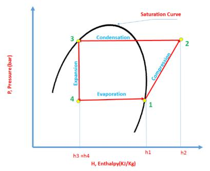
Fig. 1.1. VCR cycle on P-H diagram.
