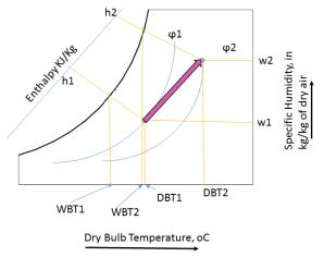
Fig. 2.6. Heating and Humidification process
