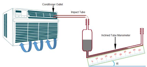
Fig. 3.3. Test set up of an air conditioner.
