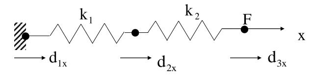
For this system of spring, first write down the total potential energy of the system as:
