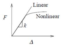
$k = F / \Delta$  (> 0) is the force needed to produce a unit stretch.
