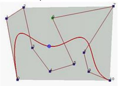
Note that not all control points are on the boundary of the convex hull. For example, control points 3, 4, 5, 6, 8 and 9 are in the interior. The curve, except for the first two endpoints, lies completely in the convex hull.
