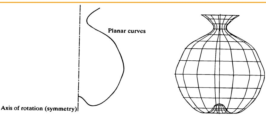
FIGURE 6-6 Surface of revolution. **Tabulated cylinder.** This is a surface generated by translating a planar curve a certain distance along a specified direction (axis of the cylinder).
