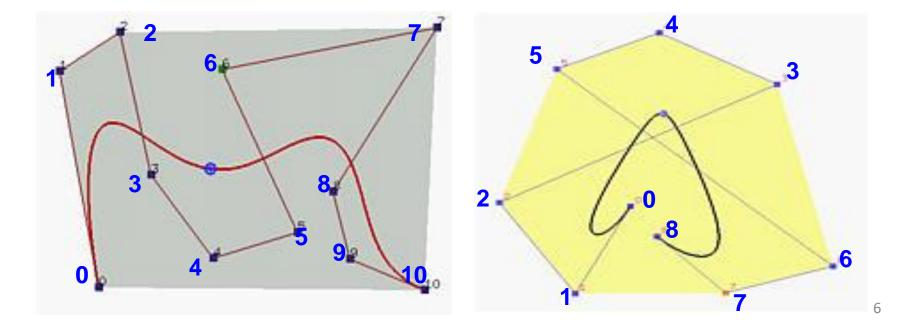
4. The Bézier curve lies completely in the **convex hull** of the given control points.
