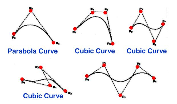
The curve passes though the first and the last control point C(u) passes through P<sub>0</sub> and P<sub>n</sub>.
