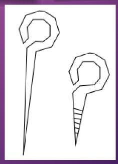
Vent rod is shown in. It is a thin spiked steel rod or wire carrying a pointed
