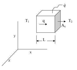
Consider the system shown above. The top, bottom, front and back of the cube are insulated, so that heat can be conducted through the cube only in the x direction. The internal heat generation per unit volume is  $\dot{q}$  (W/m<sup>3</sup>).
