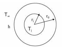
$$R_{tot} = \frac{\ln(\frac{r_0}{r_i})}{2\pi kL} + \frac{1}{(2\pi r_0 L)h}$$
