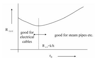
**1-D radial conduction in a sphere:**
