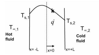
$\frac{d^2T}{dx^2} + \frac{\dot{q}}{k} = 0$ Boundary cond.: x = -L,  $T = T_{s,1}$ x = +L,  $T = T_{s,2}$ Solution:  $T = -\frac{\dot{q}}{2k}x^2 + C_1x + C_2$ Use boundary conditions to find  $C_1$  and  $C_2$ Final solution:  $T = \frac{\dot{q}L^2}{2k}\left(1 - \frac{x^2}{L^2}\right) + \frac{T_{s,2} - T_{s,1}}{2}\frac{x}{L} + \frac{T_{s,2} + T_{s,1}}{2}$
