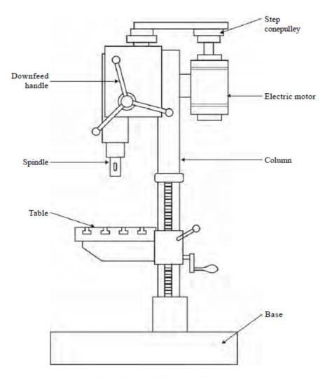
Fig 2.2 Upright drilling machine
