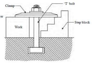
Fig 2.7 T-bolt & clamp
