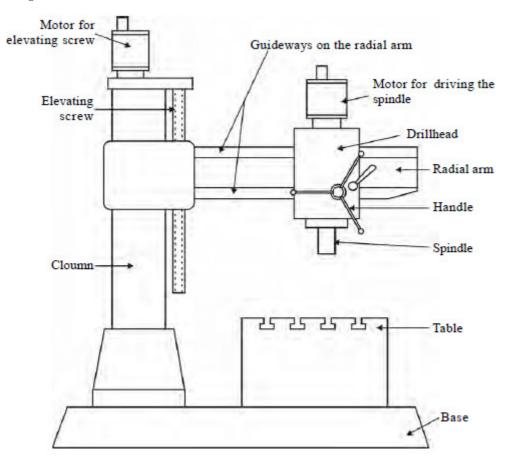
Fig 2.3 Radial drilling machine
