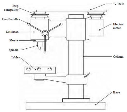
Fig 2.1 Sensitive drilling machine
