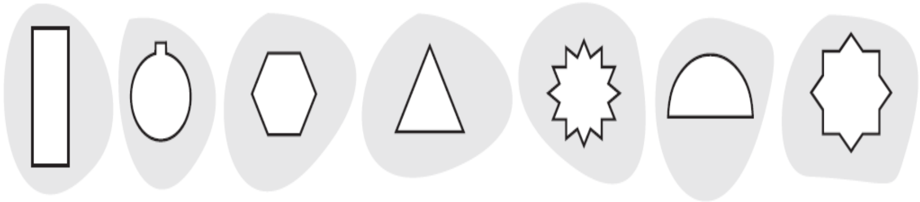
Various shapes produced by internal broaching operation.
