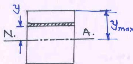
$$(\sigma_b)_{\max} = \frac{M}{I} \cdot y_{\max} \Rightarrow M = (\sigma_b)_{\max} \times \frac{I}{y_{\max}}$$
