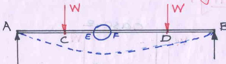
In figure shows a part of beam subjected to pure bending. The part of length  $\Delta x$  being subjected to pure bending has deformed to the shown in fig
