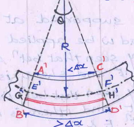
A fibre such as AC has deformed to the shape <sup>3.2</sup> A'C'. This fibre has been shortened in its length. The fibre BD on the contrary has been elongated and has taken the shape B'D'. Similarly, the fibre GH has been elongated and has taken the shape G'H'. Hence, if the beam for the length  $\Delta x$  be taken to consist of large number of fibres, we find that all of them have changed their shape: some of them have been shortened while some of them are elongated.
