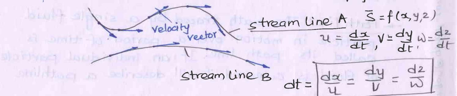
since at any point on streamline the velocity is tangential to the streamline, so the components of velocity at right angles to the streamline is always zero. Thus there can be no flow occurring across any streamline. Streamlines can not ever cross each other. If they cross the fluid particle will have two velocities at the point of intersection and that is physically impossible
