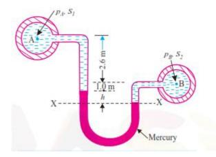
26) Fig.below shows an inverted differential manometer having an oil of specific gravity 0.8 connected to two different pipes carrying water under pressure. Determine the pressure in the pipe B. The pressure in pipe A is 2.0 metres of water.(2.22)
