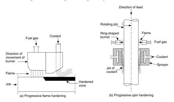
Figure 9.1 Schematic diagram illustrating two principles,
