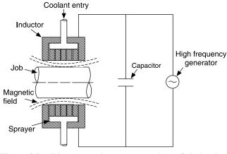
Figure 9.2 Diagrammatic representation of induction hardening process.
