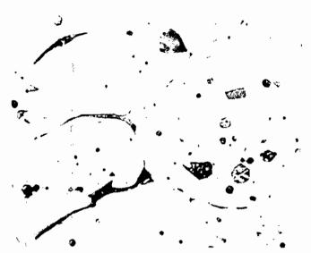
Fig. 6-13 Photomicrograph of an aluminum alloy in which some melting has occurred at the grain boundaries during heating. After cooling, these portions of the grain boundaries appear as dark broad lines; magnification, 1,000X. (Alcoa Research Laboratories, Aluminum Company of America.)
