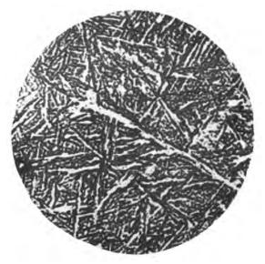
Figure 5.6 Microstructure showing coarse accicular martensite (×300).
