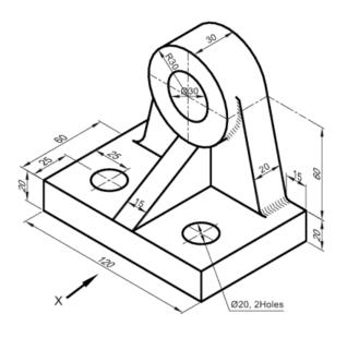
Pictorial view of a machine component is shown in Fig Draw following: (1) F.V. From X (2) T.V. and (3) Sectional LHSV from AA using Third Angle System
