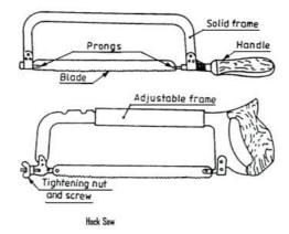
The Hack Saw is used for cutting metal by hand. It consists of a frame, which holds a thin blade, firmly in position. Hacksaw blade is specified by the number of teeth for centimeter. Hacksaw blades have a number of teeth ranging from 5 to 15 per centimeter (cm). Blades having lesser number of teeth per cm are used for cutting soft materials like aluminum, brass and bronze. Blades having larger number of teeth per centimeter are used for cutting hard materials like steel and cast Iron.
