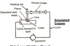
Metal-arc Welding Circuit
