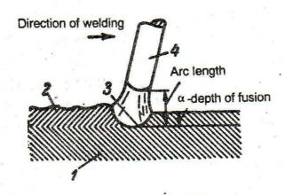
A welding arc 1. parent metal, 2. deposited metal, 3. crater, 4. electrode
