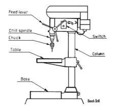
Holes are drilled for fastening parts with rivets, bolts or for producing internal thread. Bench drilling machine is the most versatile machine used in a fitting shop for the purpose. Twist drills, made of tool steel or high speed steel are used with the drilling machine for drilling holes.
