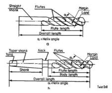
Twist drills are used for making holes. These are made of High speed steel. Both straight and taper shank twist drills are used. The parallel shank twist drill can be held in an ordinary self – centering drill check. The tapper shank twist drill fits into a corresponding tapered bore provided in the drilling machine spindle.
