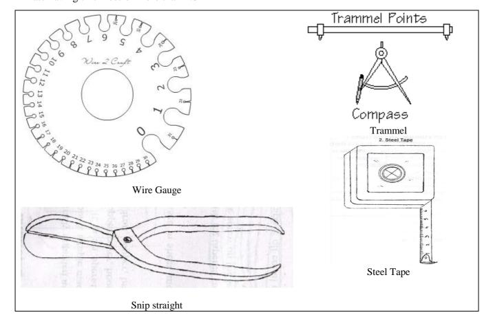
Machine used in sheet metal shop:
