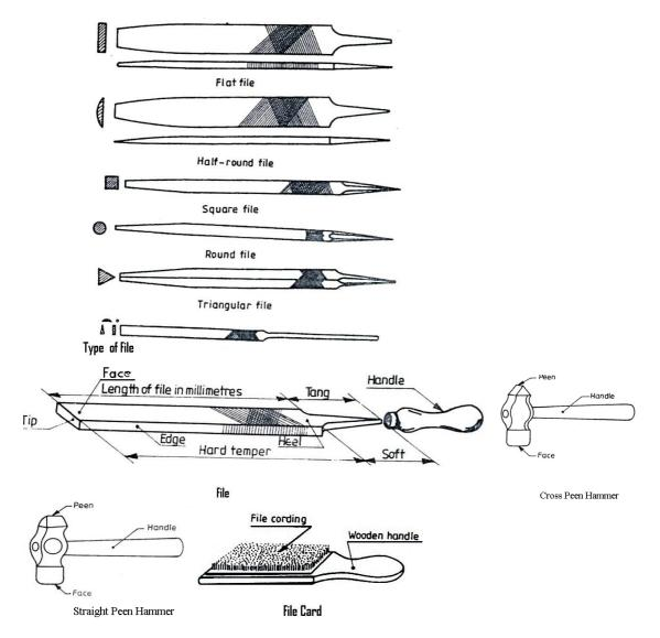
File: A file is a harden piece of high grade steel with slanting rows of teeth. Classification of files:
