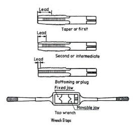
A tap is a hardened and steel tool, used for cutting internal thread in a drill hole. Hand Taps are usually supplied in sets of three in each diameter and thread size. Each set consists of a tapper tap, intermediate tap and plug or bottoming tap. Taps are made of high carbon steel or high speed steel.
