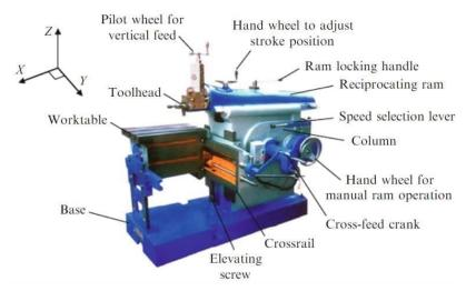
A metalworking shaper is somewhat analogous to a metalworking planer, with the cutter riding a ram that moves relative to a stationary workpiece, rather than the workpiece moving beneath the cutter. The ram is typically actuated by a mechanical crank inside the column, though hydraulically actuated shapers are increasingly used. Adding axes of motion to a shaper can yield helical tool paths, as also done in helical planing.
