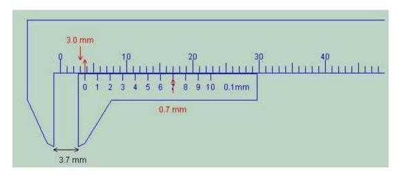
Figure 2: The reading here is 3.7 mm.
