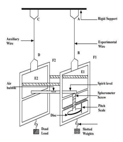
Searle's apparatus works on the principle of Hooke's law. Hooke's law can be expressed in terms of stress and strain. Stress is the force on a unit area within a material that develops as a result of the externally applied force. Strain is the relative deformation produced by stress.
