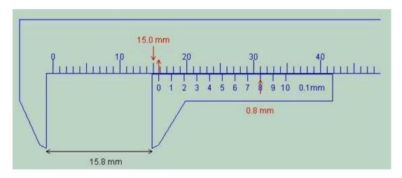
Figure 3: The reading here is 15.8 mm.
