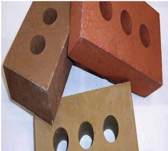
Fig.4 Green building product from fly ash Source: http://designtoimprovelife.dk/green-building-products-from-flyash/
