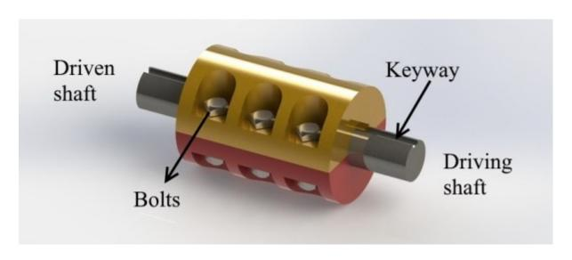
In split muff coupling, the sleeve or muff isn't a single different part instead it is split into 2
