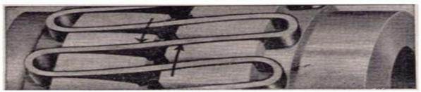
Spring condition under Severe shock load
