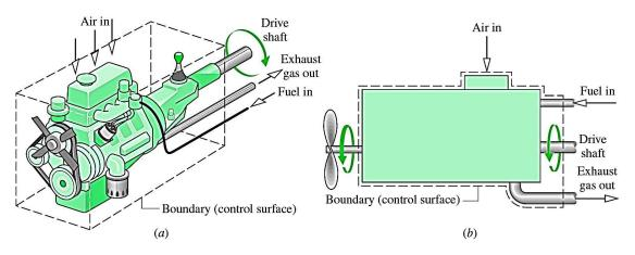
Fig. 1.10 Example of a control volume (open system) - An automobile engine
