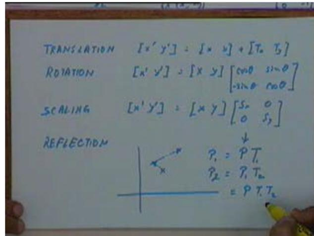
So for the four operations that we have seen we can summarize in this manner. Translation is captured by  $[x' y'] = [x y] * [T_x T_y]$ . Rotation is captured by  $[x' y'] = [x y] * \begin{bmatrix} \cos\theta & \sin\theta \\ -\sin\theta & \cos\theta \end{bmatrix}$  and
