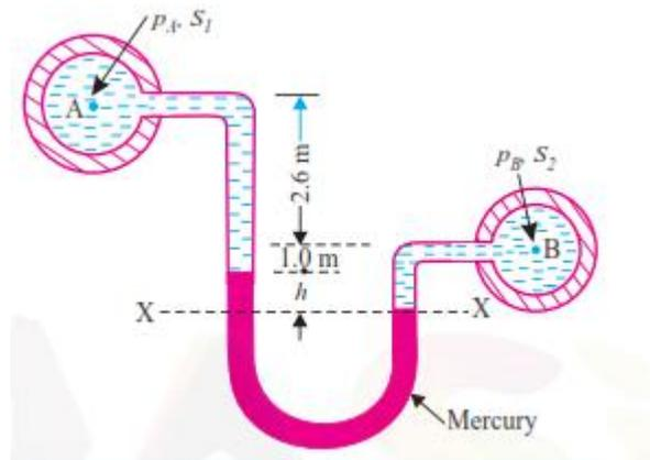
26) Fig.below shows an inverted differential manometer having an oil of specific gravity 0.8 connected to two different pipes carrying water under pressure. Determine the pressure in the pipe B. The pressure in pipe A is 2.0 metres of water.(2.22)
