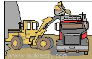
2.) Boulder-size limestone rocks are transported from the quarry to the cement plant and fed into a crusher which crushes the boulders into marble-size pieces.
