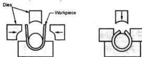
Fig. 15: Bending in a 4-slide machine
