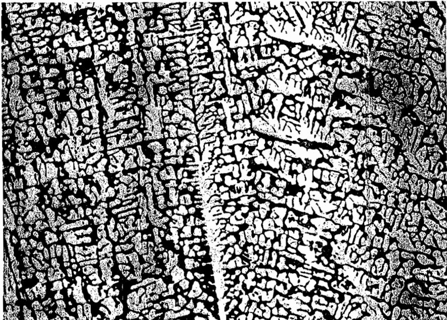
Fig. 6-10 Fine-cored dendrites in a copper-lead alloy; magnification 100X. (Research Laboratories, National Lead Company.)
