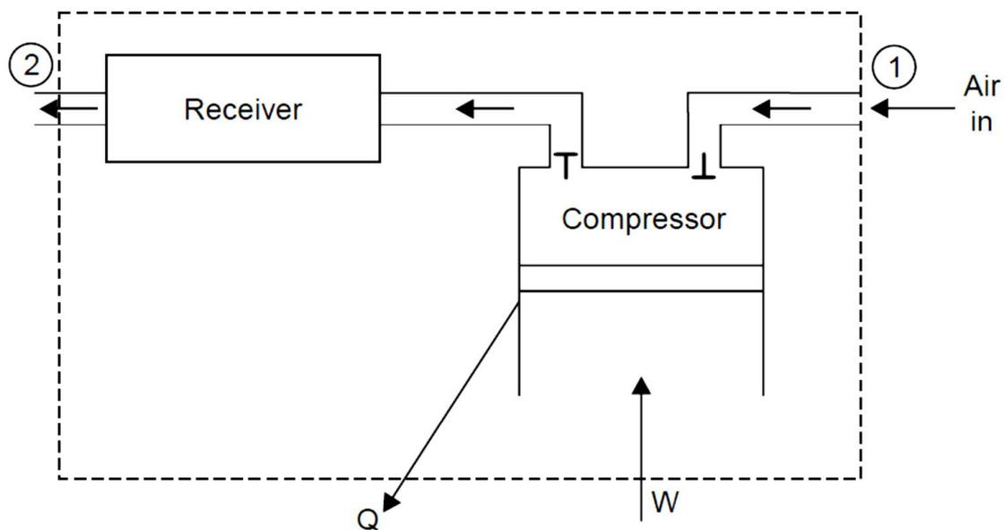
Fig. 2.10 Schematic of reciprocating compressor
