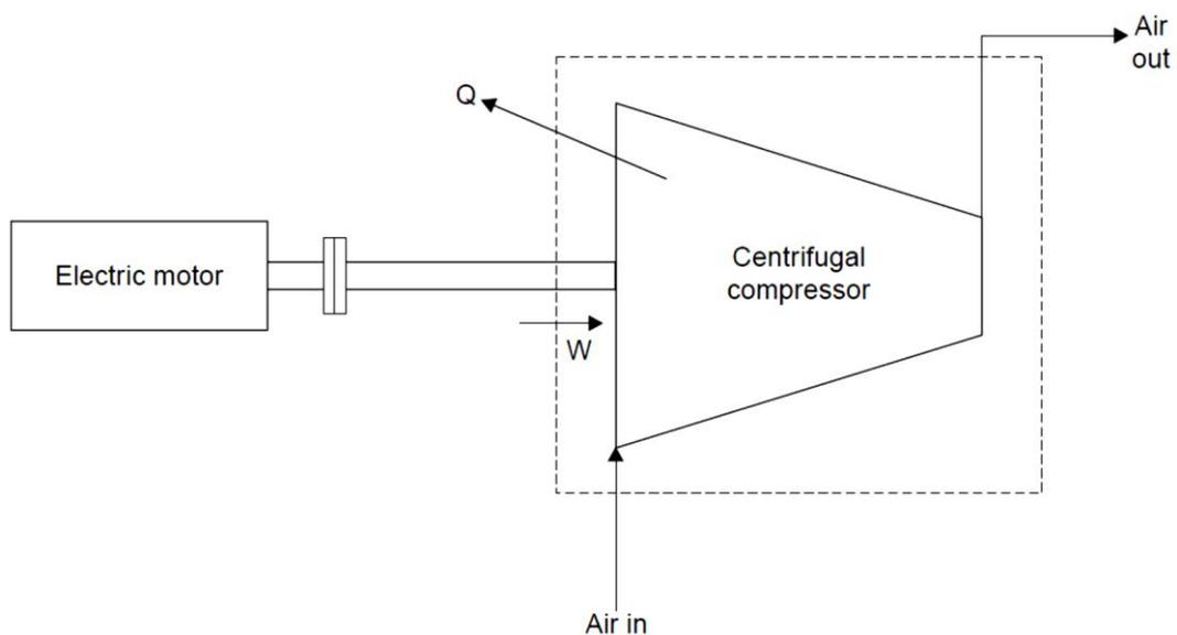
Fig. 2.11 Schematic of rotary compressor
