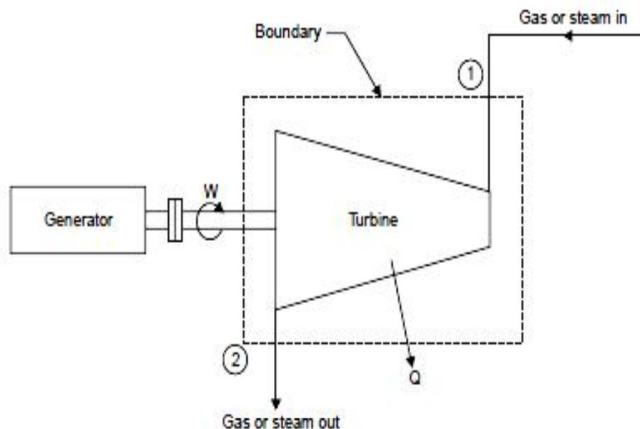
Fig. 2.7 Schematic of steam or gas turbine
