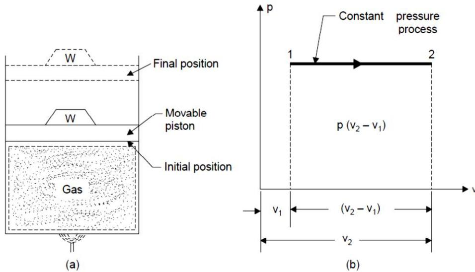
Fig. 2.16 Constant pressure process (Isobaric)
