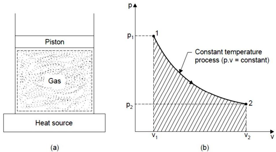
Fig. 2.17 Constant temperature process (Isothermal)
