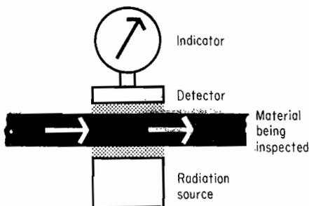
Fig. 1-30 A simple radiation thickness gauge.
