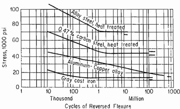
Fig. 1-27 Typical *S-N* (stress-cycle) diagrams. (From "Metals Handbook," 1948 ed., American Society for Metals, Metals Park, Ohio.)
