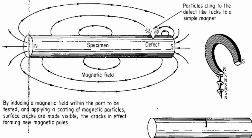
By inducing a magnetic field within the part to be tested, and applying a coating of magnetic particles, surface cracks are made visible, the cracks in effect forming new magnetic poles
