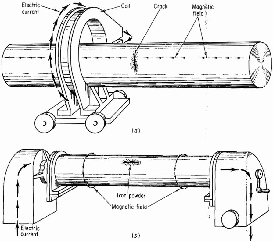
Fig. 1-32 Illustrating two kinds of magnetization: (a) Longitudinal magnetization; (b) circular magnetization. (Magnaflex Corporation, Chicago, Ill.)
