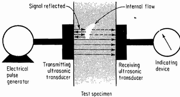
Fig. 1-36 The through-transmission and pulse-echo methods of ultrasonic inspection.
