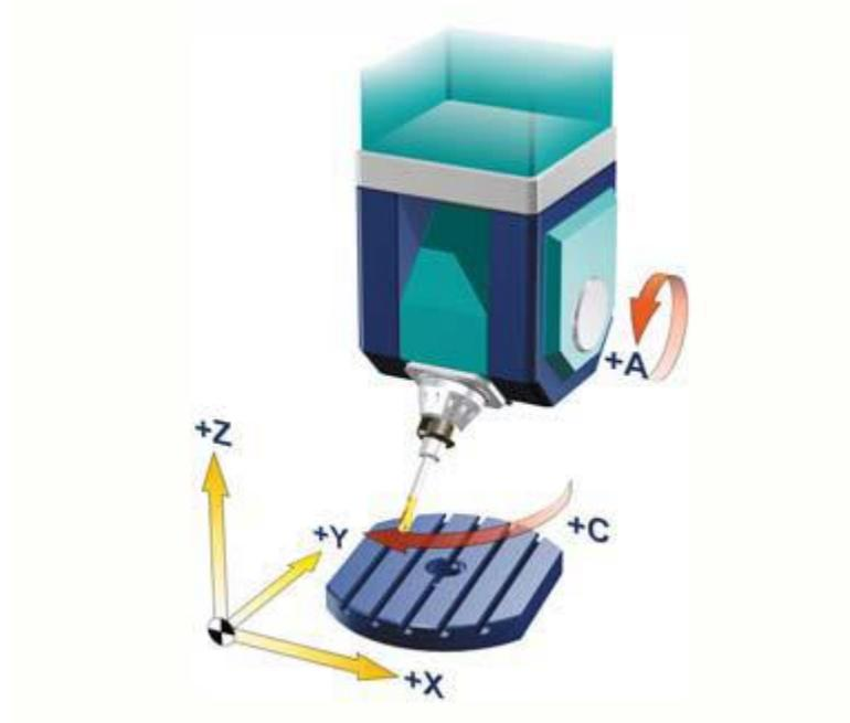
One rotary axis in head / one rotary axis
