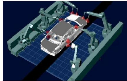
In the paint shop, flexibility means robotic applicators are programmed to cover various body styles – as they move through the paint booth – with equal precision. This results in minimizing waste and environmental impact while maximizing quality.
