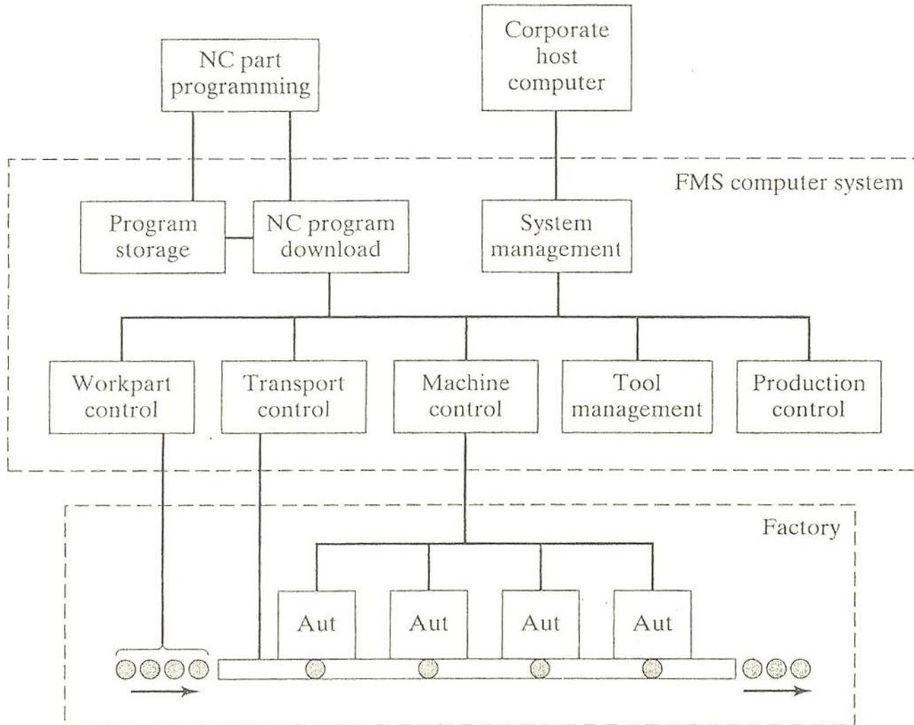
**Figure 16.11** Structure of FMS application software system. Key: NC = numerical control, Aut = automated workstation.
