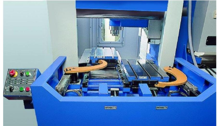
Machining Center with Pallet changer
