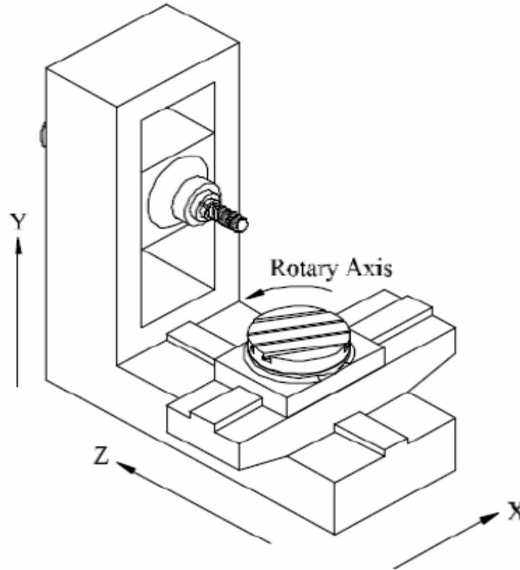
4-Axis Machining Center (HMC)
