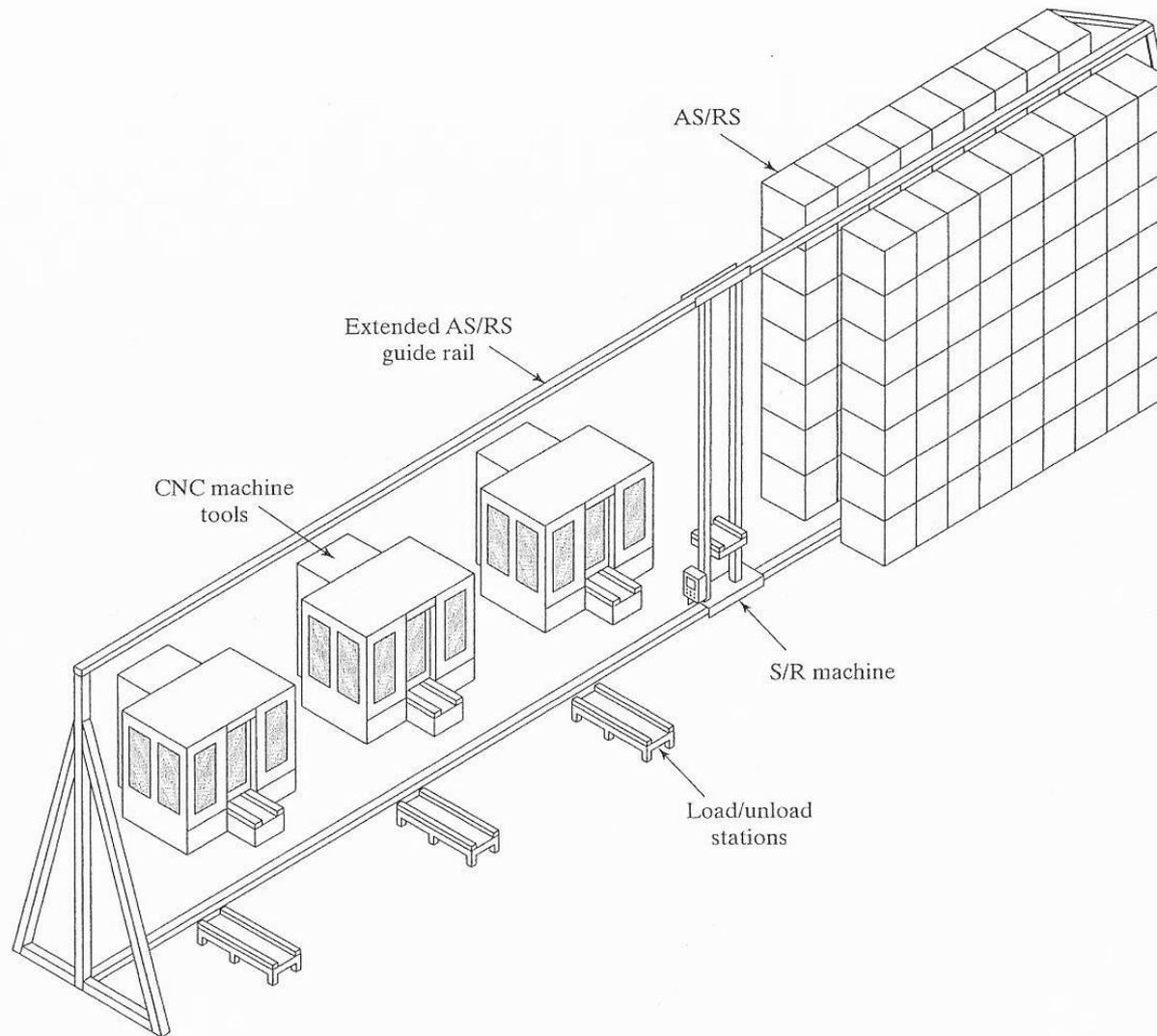
**Figure 16.6** FMS that incorporates an automated storage and retrieval system for handling and storing parts. Key: AS/RS = automated storage/retrieval system, S/R = storage/retrieval machine (also known as a stacker crane), CNC = computer numerical control.
