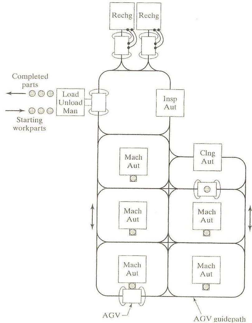
**Figure 16.10** Open field FMS layout. Key: Load = parts loading, UnLd = parts unloading, Mach = machining, Clng = cleaning, Insp = inspection, Man = manual, Aut = automated, AGV = automated guided vehicle, Rechg = battery recharging station for AGVs.
