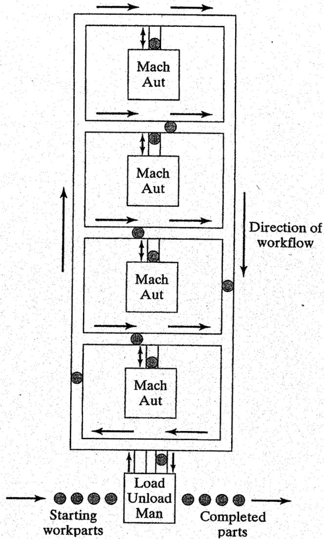
**Figure 16.9** FMS ladder layout. Key: Load = parts loading station, UnLd = parts unloading station, Mach = machining station, Man = manual station, Aut = automated station.
