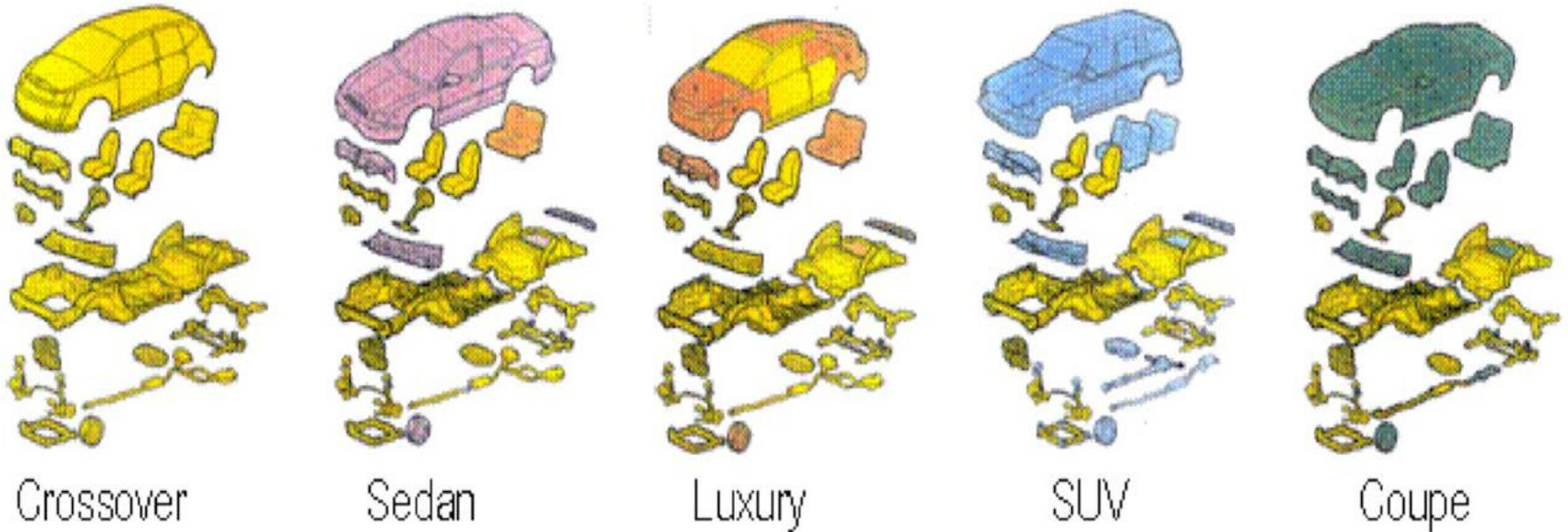
When different models are designed to be assembled in the same sequence they can be built in the same plant.
