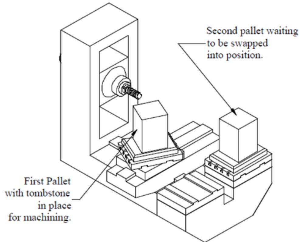
Machining Center with Pallet changer
