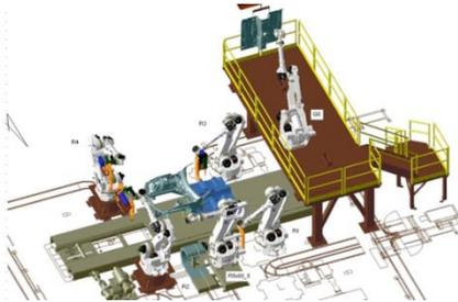
In the body shop, where the sheet metal comes together to form the vehicle's body, flexibility means more than 80 percent of the tooling is not specific to one model. It can be reprogrammed to weld a car or a truck or a crossover of similar size.
