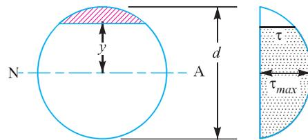
Fig. 5.31. Shear stress in a circular beam.
