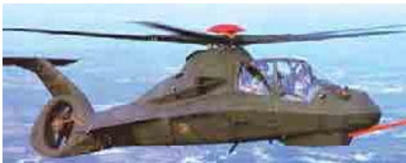
*This picture shows a reconnaissance helicopter of air force. Its dark complexion absorbs light that falls on its surface. The flat and sharp edges deflect radar waves and they do not return back to the radar. These factors make it difficult to detect the helicopter.*
