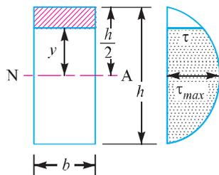
Fig. 5.30. Shear stress in a rectangular beam.
