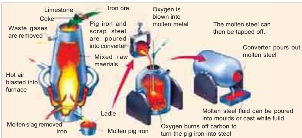
Pig iron is made from iron ore in a blast furnace. It is a brittle form of iron that contains 4-5 per cent carbon.
