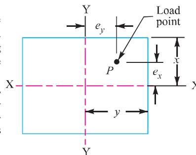
**Fig. 5.20.** Eccentric load with eccentricity about two axes.
