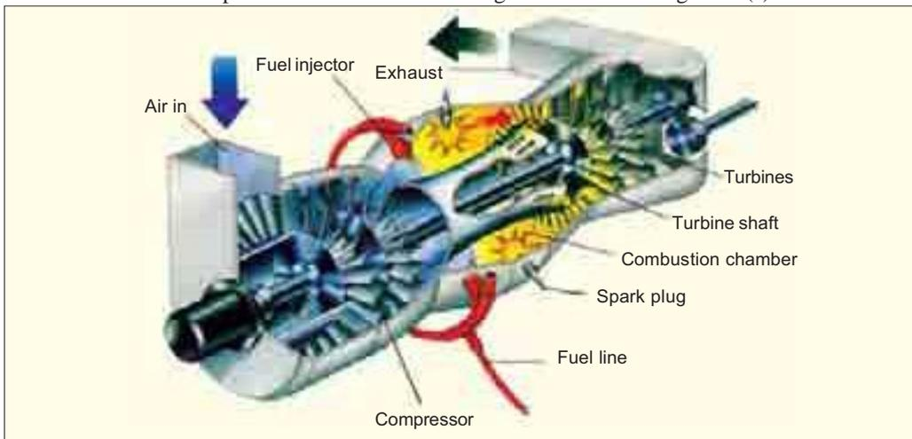
In a gas-turbine system, a compressor forces air into a combustion chamber. There, it mixes with fuel. The mixture is ignited by a spark. Hot gases are produced when the fuel burns. They expand and drive a series of fan blades called a turbine.
