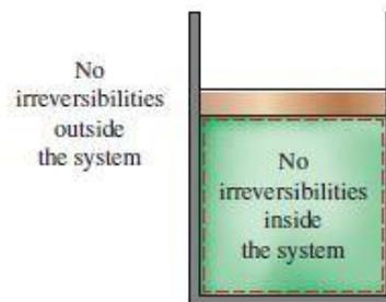
Fig.3.23 - A reversible process involves no internal and external irreversibilities.
