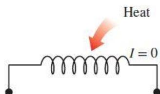
*Fig.3.2 - Transferring heat to a wire will not generate electricity*
