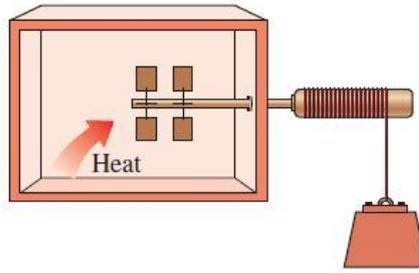
Fig.3.3 - Transferring heat to a paddle wheel will not cause it to rotate
