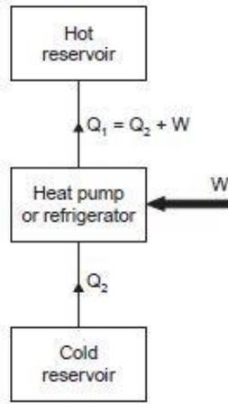
Fig.3.9 – Heat pump or Refrigerator
