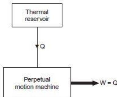
Fig.3.10 - Perpetual motion machine of second kind (PMM2)
