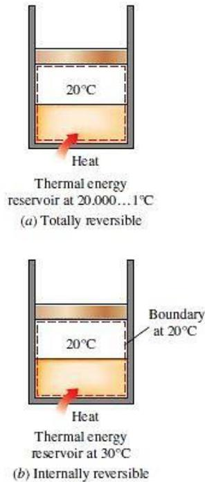
Fig.3.24 - Totally and internally reversible heat transfer processes.
