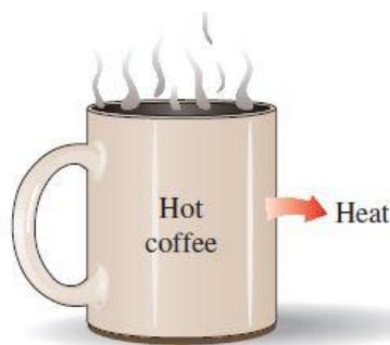
*Fig.3.1 - A cup of hot coffee does not get hotter in a cooler room*
