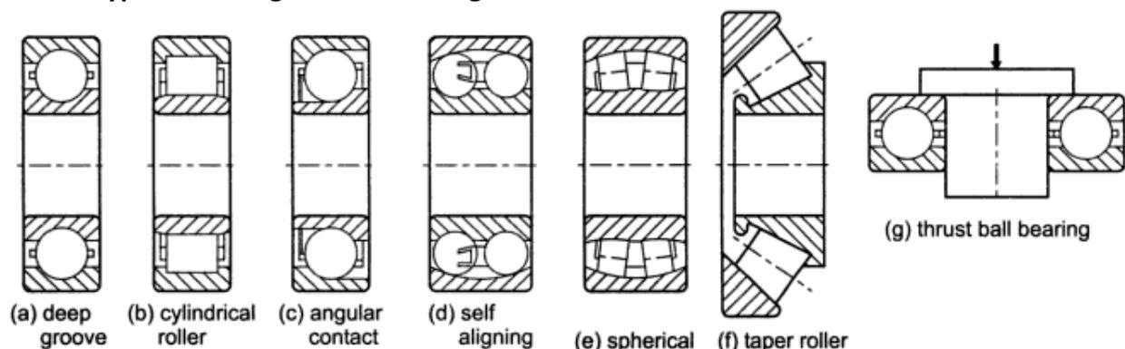
*Fig. 4.1 Types of Rolling Contact Bearings*
