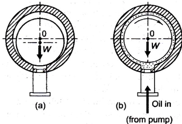
*Fig. 3.6 Hydrostatic Lubrication (a) Journal at Rest
