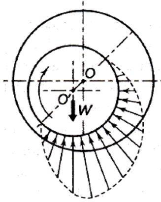
*Fig. 3.4 Pressure Distribution in Hydrodynamic Bearing*
