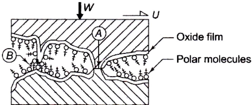
*Fig. 3.7 Boundary Lubrication: (a) Metal to Metal Contact (b) Cluster of Molecules*
