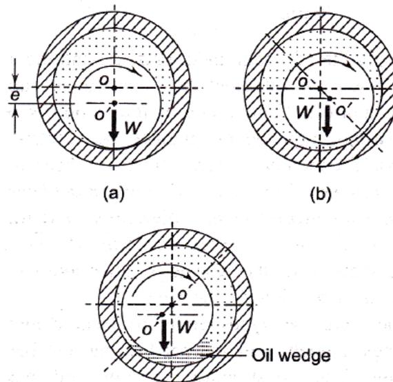
*Fig. 3.3 Hydrodynamic Lubrication (a) Journal at Rest
