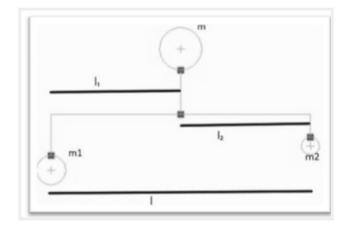
In the given figure,m1=10, Kg m2=30Kg and m=50 Kg, if r1=0.2m and r=0.3m, I=1m, find I2. \* (3 Points)
