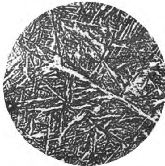
**Figure 5.6** Microstructure showing coarse accicular martensite ( $\times 300$ ).
