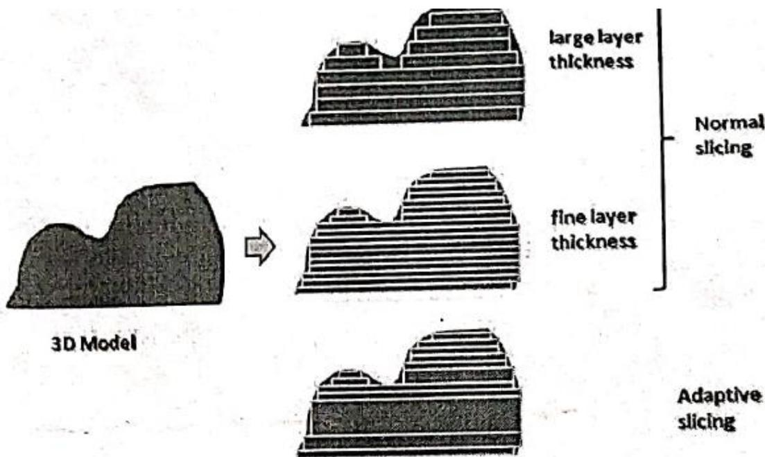
Figure 7.3 normal slicing and adaptive slicing
