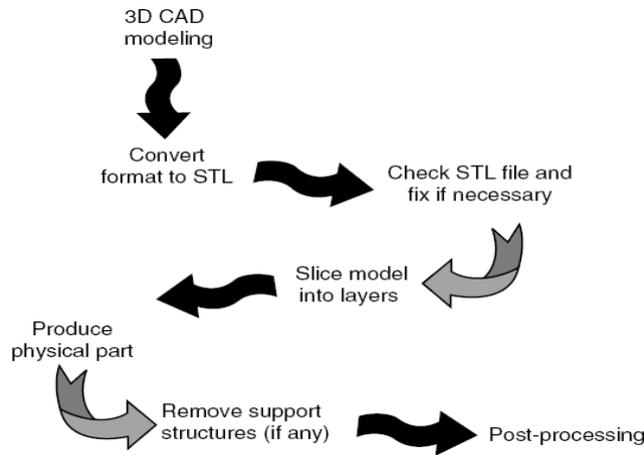
Fig. 1.5 Data Flow of the Basic RP Process
