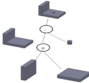
**Fig. 1.3 Constructive Solid Geometry**
