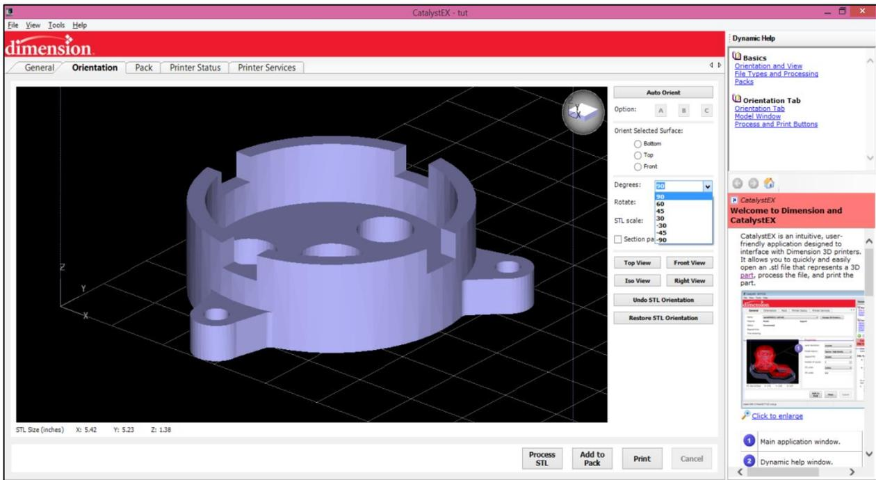
Figure 4.7 selection of manual orientation at diff. degree
