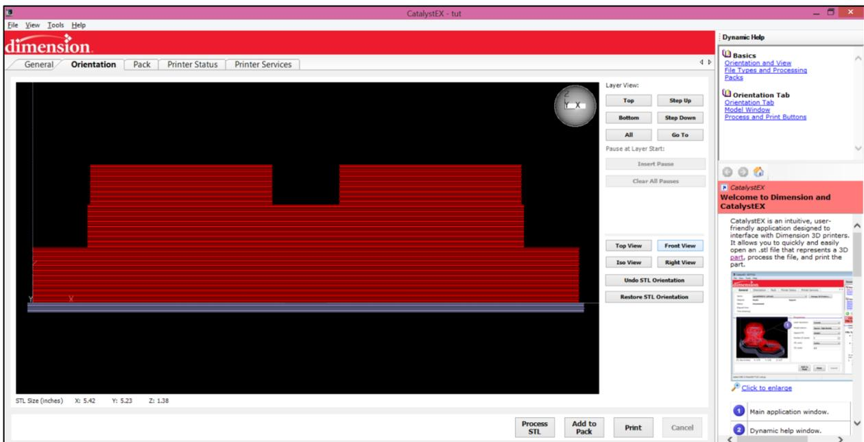
Figure 4.8 Layer thickness of 0.01 inch throughout the part
