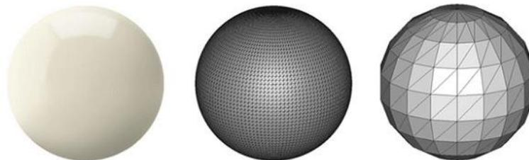
**Fig 2.3 - Effect of degree of approximation in tessellation on Solid geometry**
