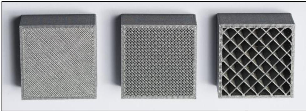
Fig. 3.3 (A) solid (B) sparse high density (C) sparse low density
