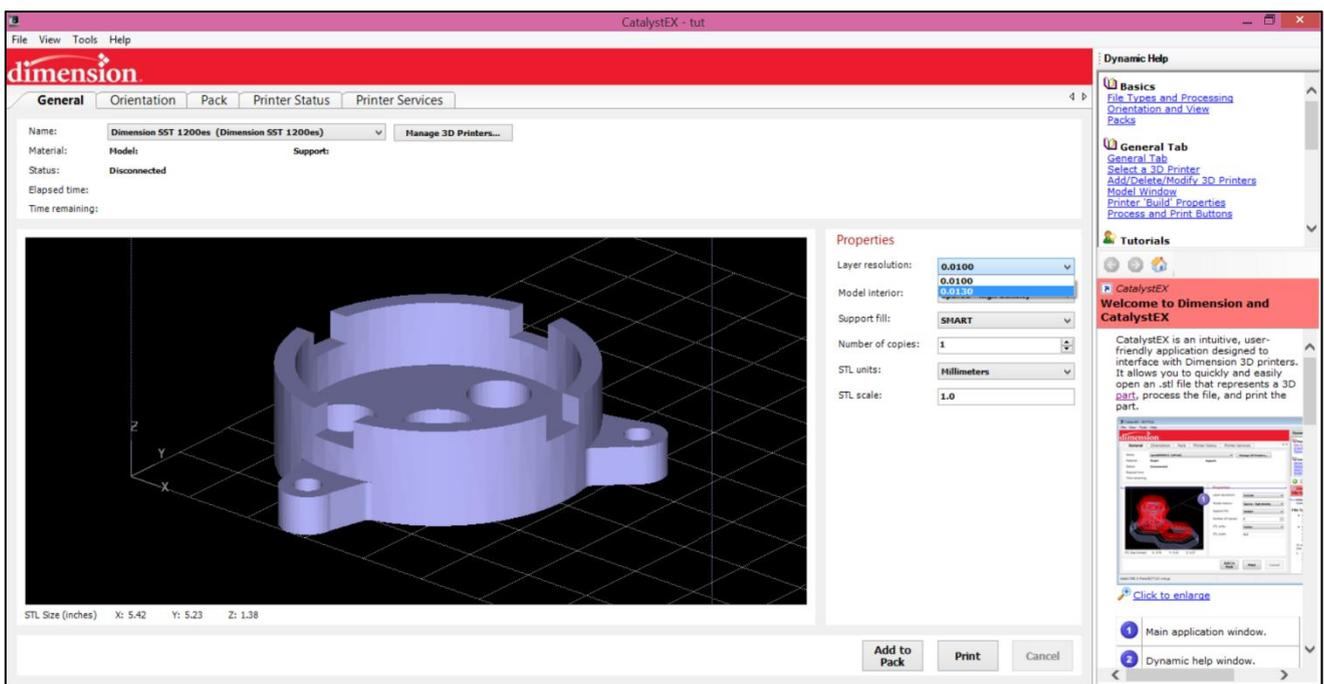
Figure 4.1 selection of layer thickness
