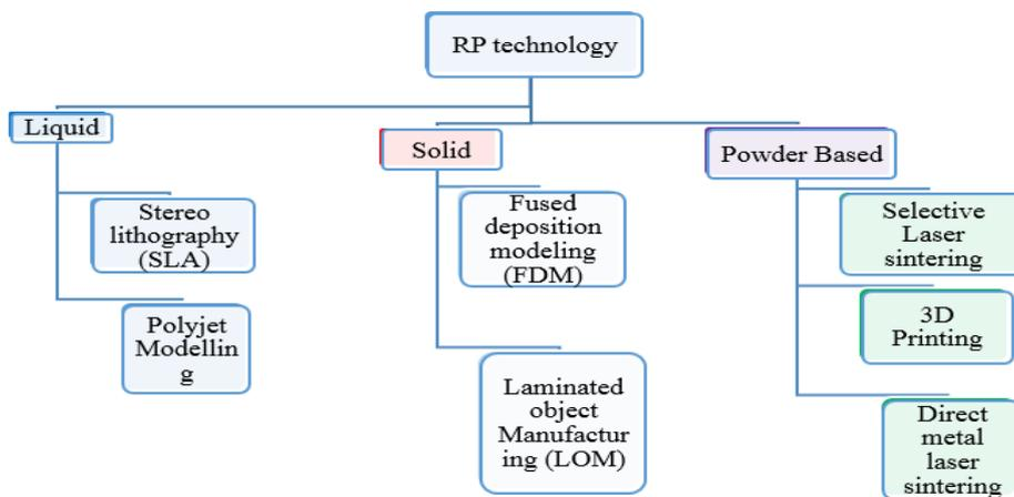
Fig. 1.6 Classification of Rapid Prototyping Systems
