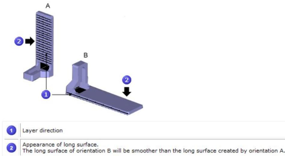
4. **STL File Repair** - It is possible for an STL file to have errors while appearing to be trouble free. If the STL file contains errors, Catalyst EX may have problems processing the file. Catalyst EX has the ability to automatically correct some STL file errors. How the part is oriented can impact this automated repair function.
