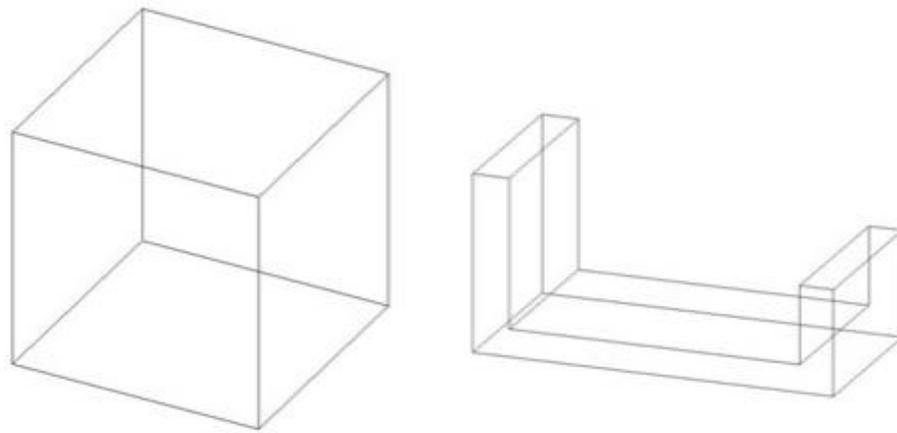
**Fig. 1.1 Wire frame model**
