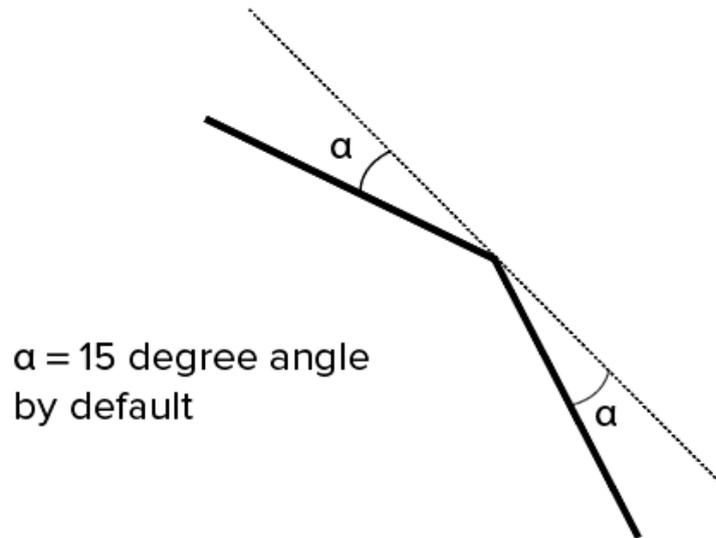
**Fig 2.5- Angular tolerance (Angle between the normal of adjacent triangles )**
