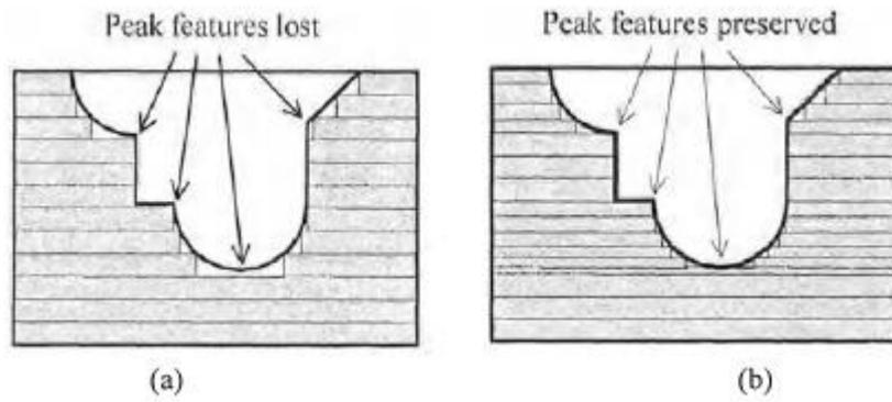
**Figure 7.5 (a) peak features lost with uniform slicing; (b) peak feature preserved with adaptive slicing**
