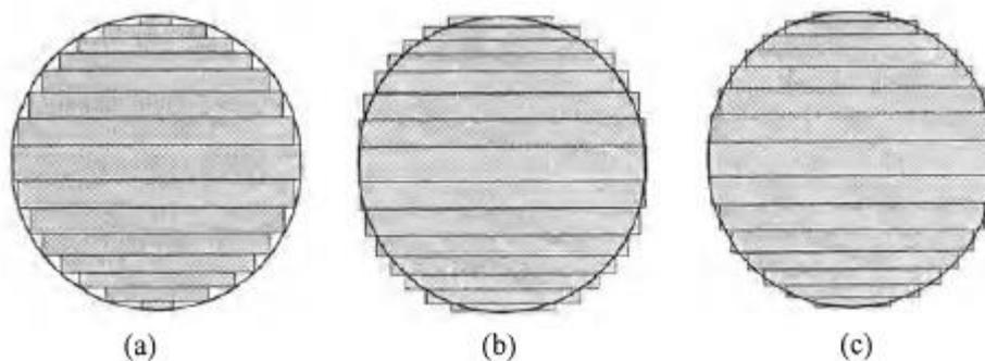
**Figure 7.4: a) negative tolerance b) positive tolerance c) mixed tolerance**
