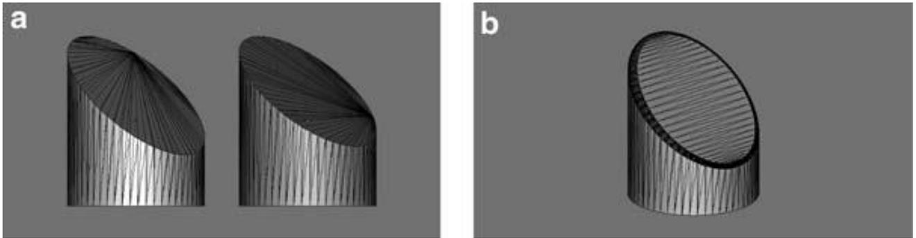
**Fig 2. 6- STL files of a cut cylinder.**
