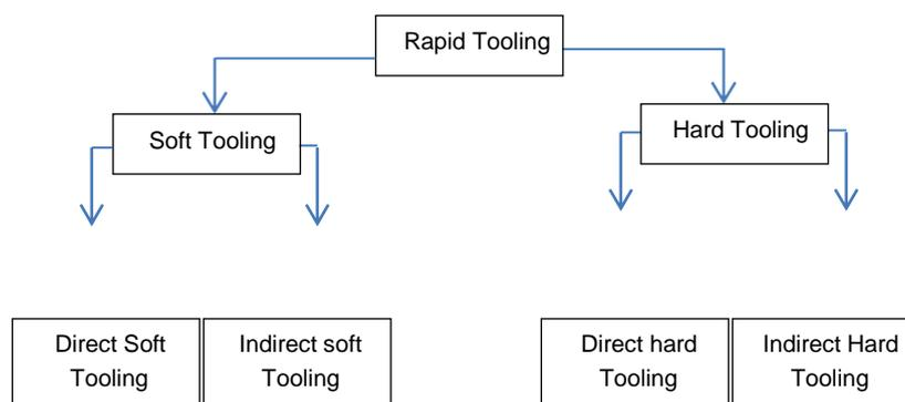
**Fig.1.7 Classification of Rapid Tooling**
