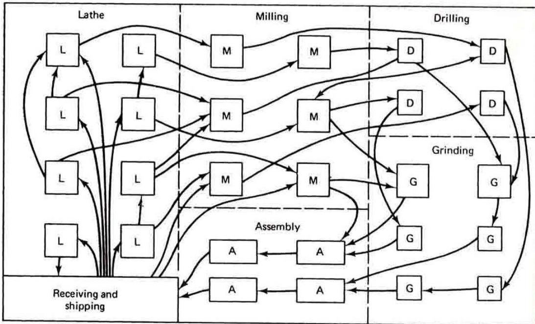
Fig.4.3 - Process-type layout
