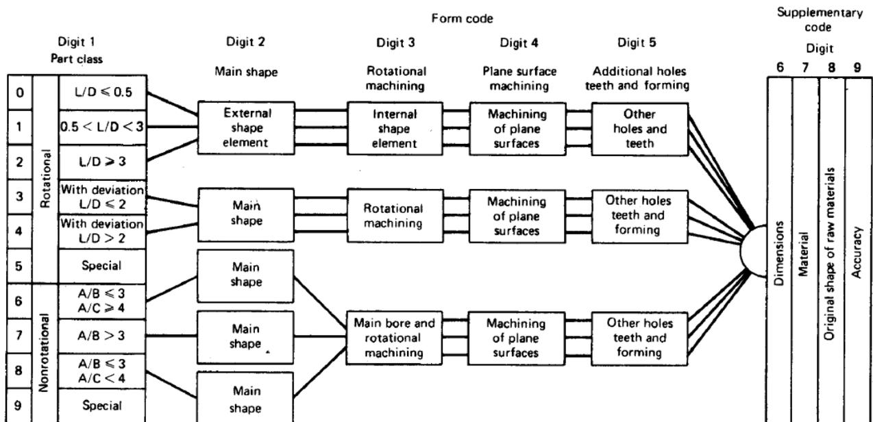
Fig.4.5 - Basic structure of the Opitz system
