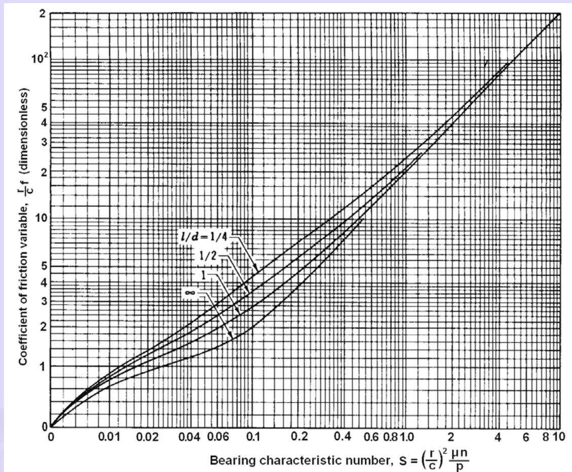
**Fig. 2.11 Chart for coefficient of friction variable.**
