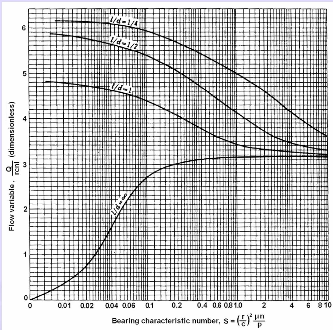
**Fig. 2.12 Chart for flow variable.**
