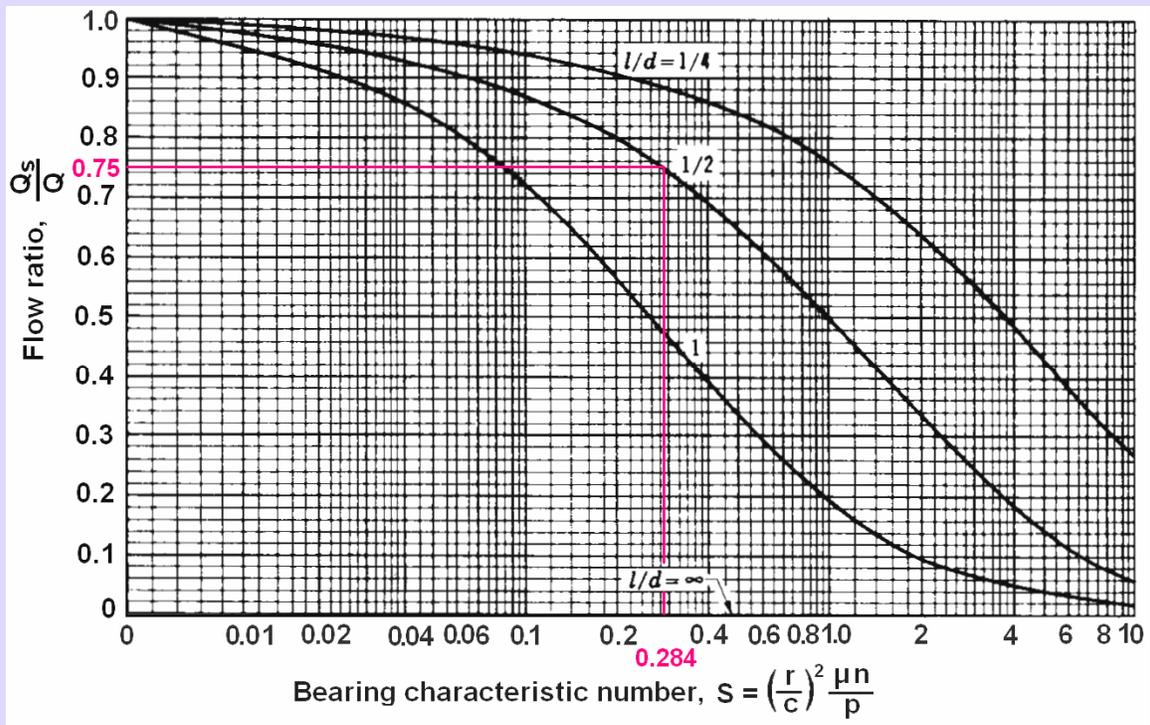
**Fig.2.13a Chart for determining the ratio of side flow to total flow**
