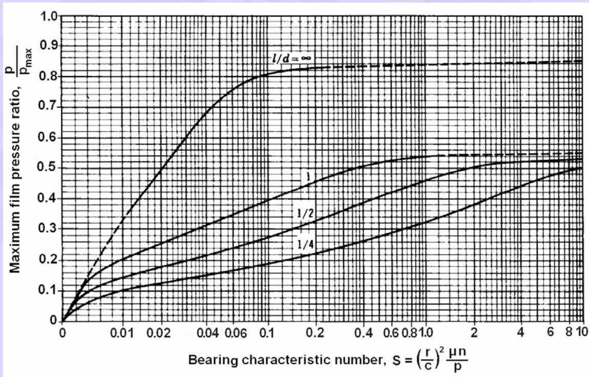
**Fig. 2.14** Chart for determining the maximum film pressure.
