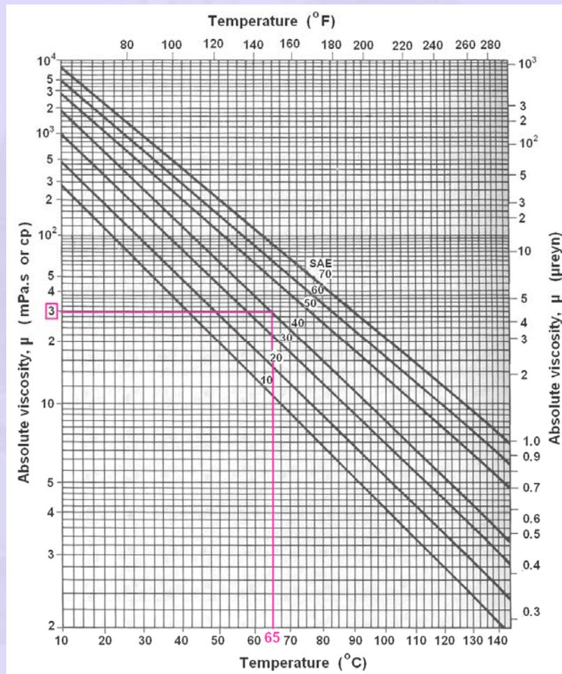
**Fig.2.3a Viscosity – temperature curves of SAE graded oils**
