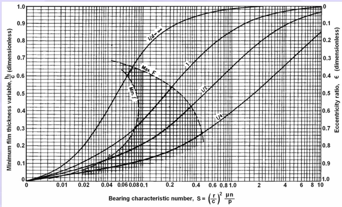
**Fig.2.8 Chart for minimum film thickness variable and eccentricity ratio. The left shaded zone defines the optimum  $h_0$  for minimum friction; the right boundary is the optimum  $h_0$  for maximum load**
