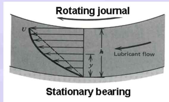
**Fig. 2.7 Velocity gradient in the oil film**
