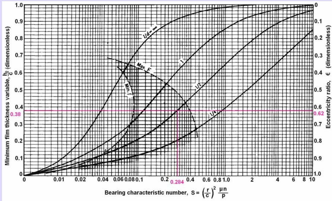
**Fig.2.8a Chart for minimum film thickness variable and eccentricity ratio.** The left shaded zone defines the optimum  $h_0$  for minimum friction; the right boundary is the optimum  $h_0$  for maximum load
