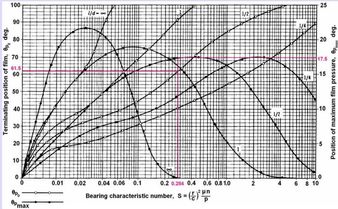
**Fig. 2.15a** Chart for finding the terminating position of oil film and position of maximum film pressure
