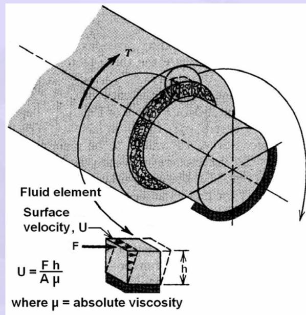
**Fig. 2.2 Laminar flow of fluid in clearance space**
