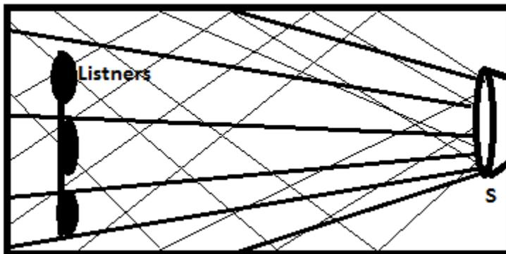
Sound undergoes by a multiple reflection by walls, floor and ceiling and directly towards the listners which produce reverberation effect.
