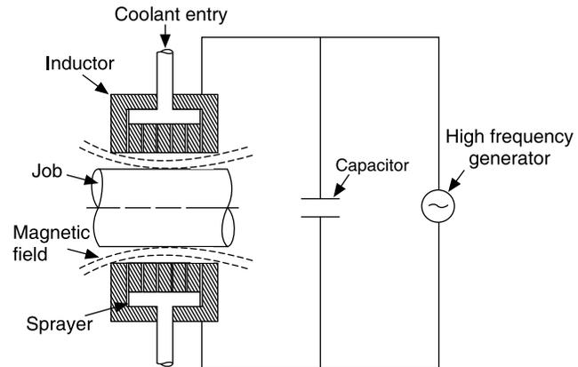
**Figure 9.2 Diagrammatic representation of induction hardening process.**
