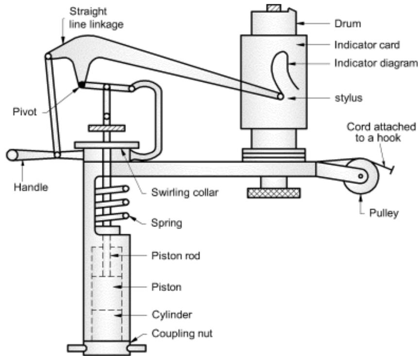
*Fig. 5. 1 Engine indicator (Mechanical type)*
