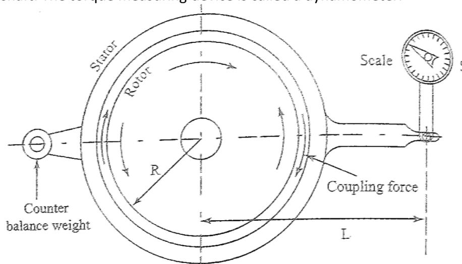
Fig. 5. 2 Principle of a dynamometer
