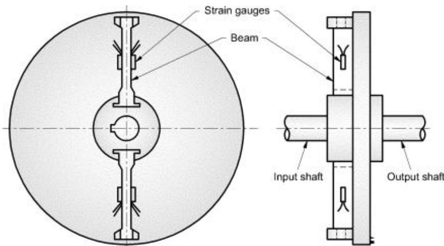
Fig. 5. 7 Transmission dynamometers
