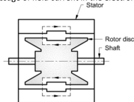
*Fig. 5. 6 Eddy current dynamometer*
