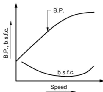
Fig. 5.15 Performance curve for CI engine
