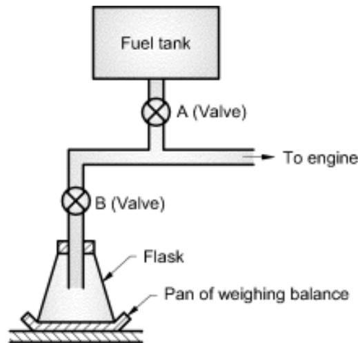
Fig. 5. 11 Direct weighing of fuel flow
