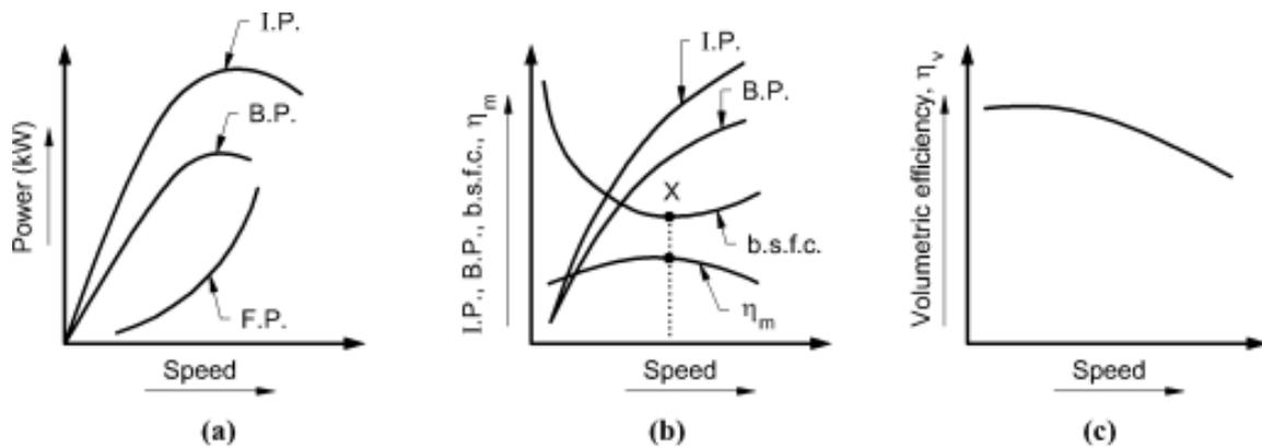
Fig. 5.14 Performance curve for S.I. engine
