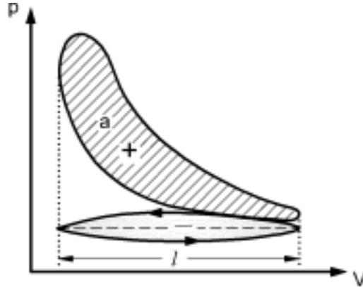
Fig. 5. 2 Indicator diagram
