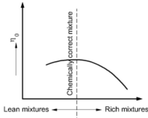
Fig. 5. 17 Brake thermal Vs Mixture strength
