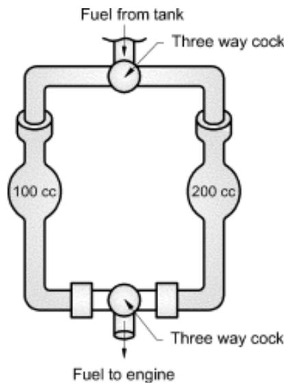
*Fig.5.10 Volumetric Type Fuel Flow meter*
