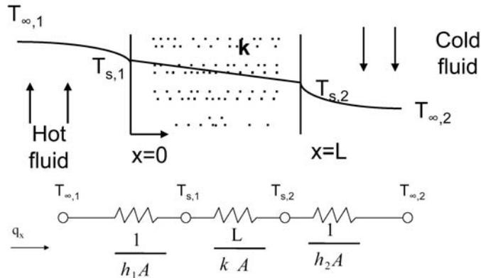
The heat transfer rate may be determined from separate consideration of each element in the network. Since  $q_x$  is constant throughout the network, it follows that
