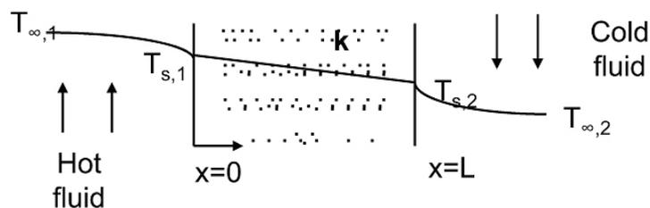
The differential equation governing heat diffusion is:  $\frac{d}{dx} \left( k \frac{dT}{dx} \right) = 0$
