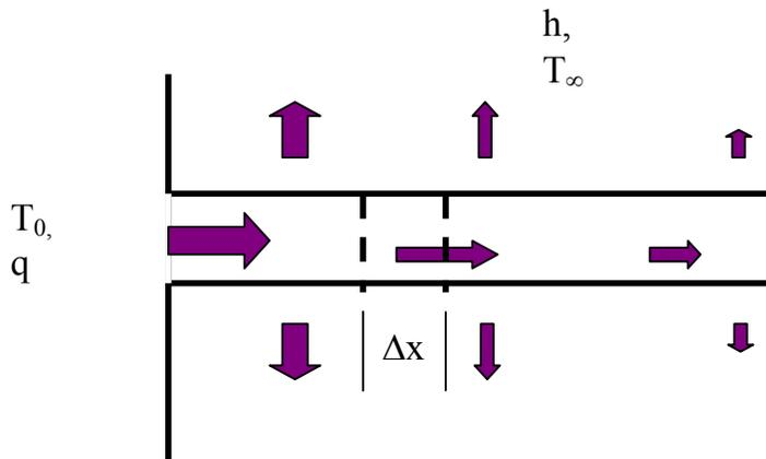
Across this segment the heat loss will be  $h \cdot (P \cdot \Delta x) \cdot (T - T_\infty)$ , where  $P$  is the perimeter around the fin. The equivalent heat sink would be  $\ddot{q} \cdot (A_c \cdot \Delta x)$ .
