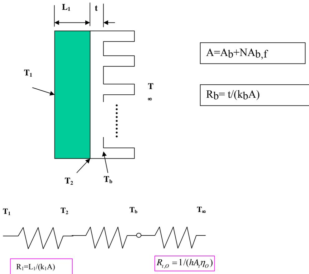
$$q = \frac{T_1 - T_\infty}{\sum R} = \frac{T_1 - T_\infty}{R_1 + R_b + R_{t,o}}$$
