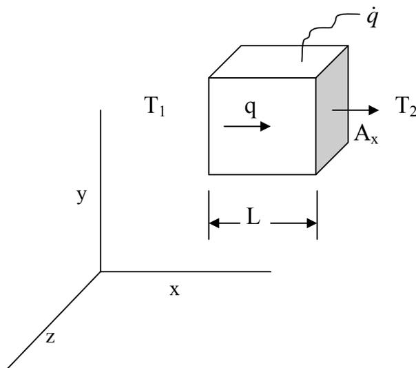
Consider the system shown above. The top, bottom, front and back of the cube are insulated, so that heat can be conducted through the cube only in the  $x$  direction. The internal heat generation per unit volume is  $\dot{q}$  ( $\text{W}/\text{m}^3$ ).
