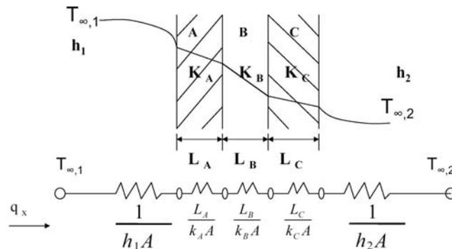
The steady state heat flow rate through the walls is given by:
