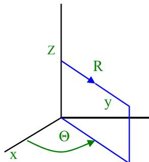
$$\frac{1}{a} \cdot \frac{\partial T}{\partial \tau} = \frac{1}{r} \frac{\partial}{\partial r} \left( r \cdot \frac{\partial T}{\partial r} \right) + \frac{1}{r^2} \cdot \frac{\partial^2 T}{\partial \theta^2} + \frac{\partial^2 T}{\partial z^2} + \frac{\dot{q}}{k}$$
