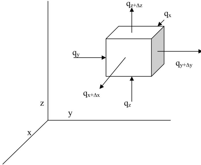
In the equation above we substitute the 6 heat inflows/outflows using the appropriate sign:
