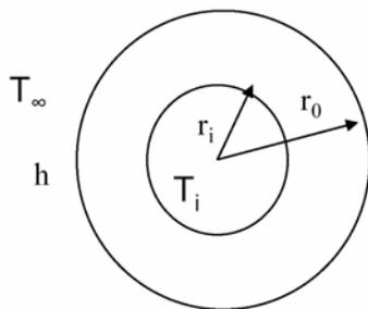
$$R_{tot} = \frac{\ln \left( \frac{r_o}{r_i} \right)}{2\pi kL} + \frac{1}{(2\pi r_o L)h}$$
