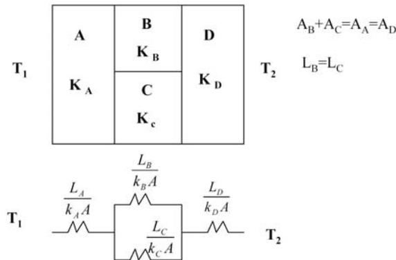
The following assumptions are made with regard to the above thermal resistance model:
