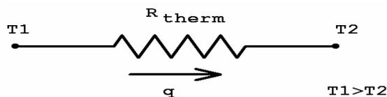
A thermal resistance may also be associated with heat transfer by convection at a surface. From Newton's law of cooling,
