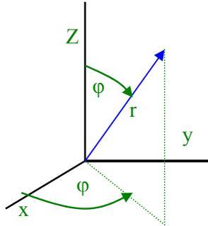
$$\frac{1}{a} \cdot \frac{\partial T}{\partial \tau} = \frac{1}{r^2} \frac{\partial}{\partial r} \left( r^2 \cdot \frac{\partial T}{\partial r} \right) + \frac{1}{r^2 \cdot \sin^2 \theta} \cdot \frac{\partial^2 T}{\partial \phi^2} + \frac{1}{r^2 \sin \theta} \cdot \frac{\partial}{\partial \theta} \left( \sin \theta \cdot \frac{\partial T}{\partial \theta} \right) + \frac{\dot{q}}{k}$$
